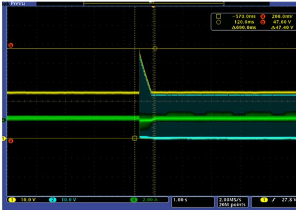
Figure 8. VM Pumping When PWM Reduces from 100% to 50% (with Ts1 on Figure 5)
