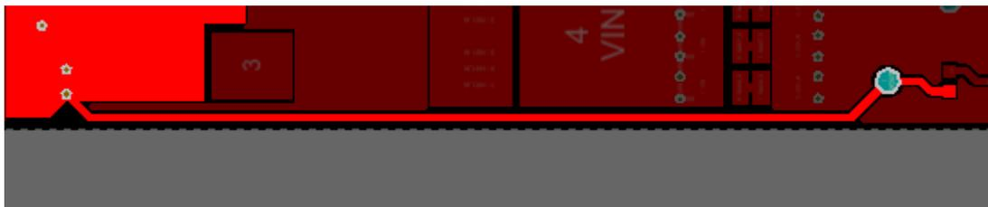
**Figure 2. Feedback Trace Routed along the Edge of the Board to Avoid Noisy Switch Nodes**
