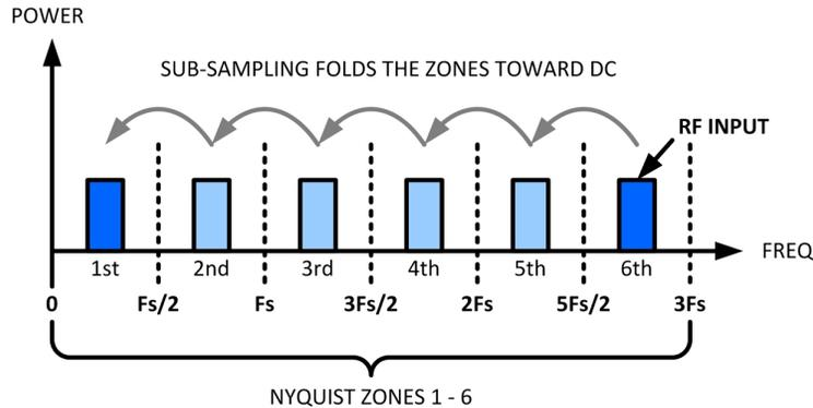
**Figure 2. Higher-order Frequency Components Are Folded into the Lower Nyquist Zones When Subsampling**
