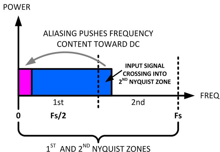
**Figure 1. The Input Signal Crosses into the Second Nyquist Zone and Is Aliased into the Signal's Operating Band**
