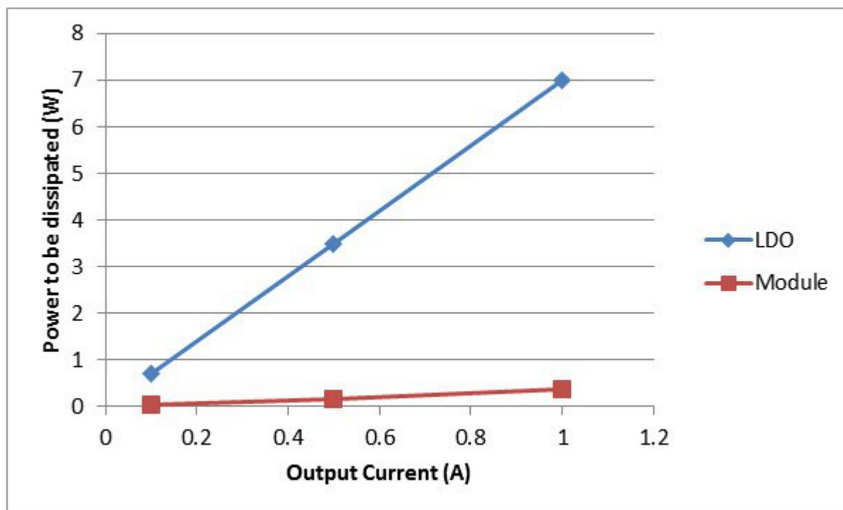
**Figure 2. Power Dissipated by a LDO and a DC/DC Switch-mode Power Supply versus Output Current**
