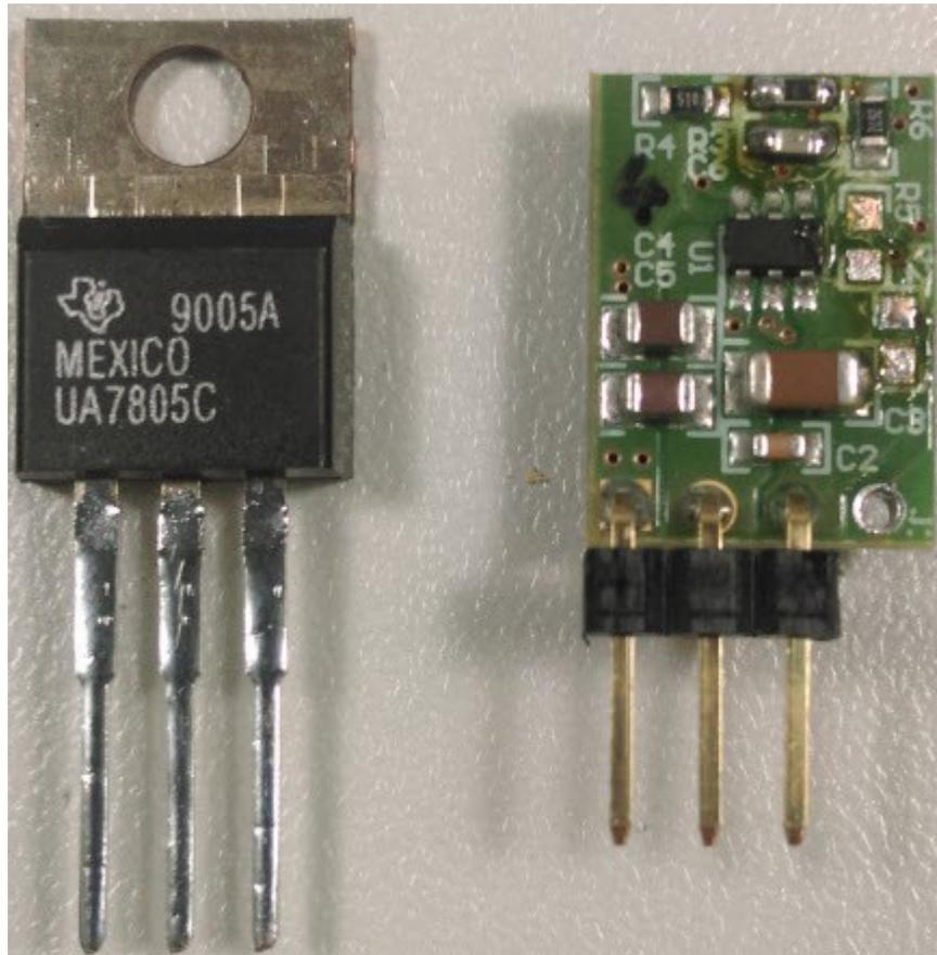
**Figure 1. High-efficiency 5V, 1A Switch-mode Power Supply Design in a T0-220 Form Factor**
