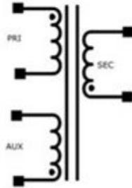
**Transformer Construction Diagram**
