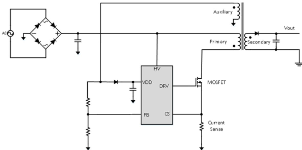
**Figure 2. AC/DC Flyback with Primary-side Regulation**
