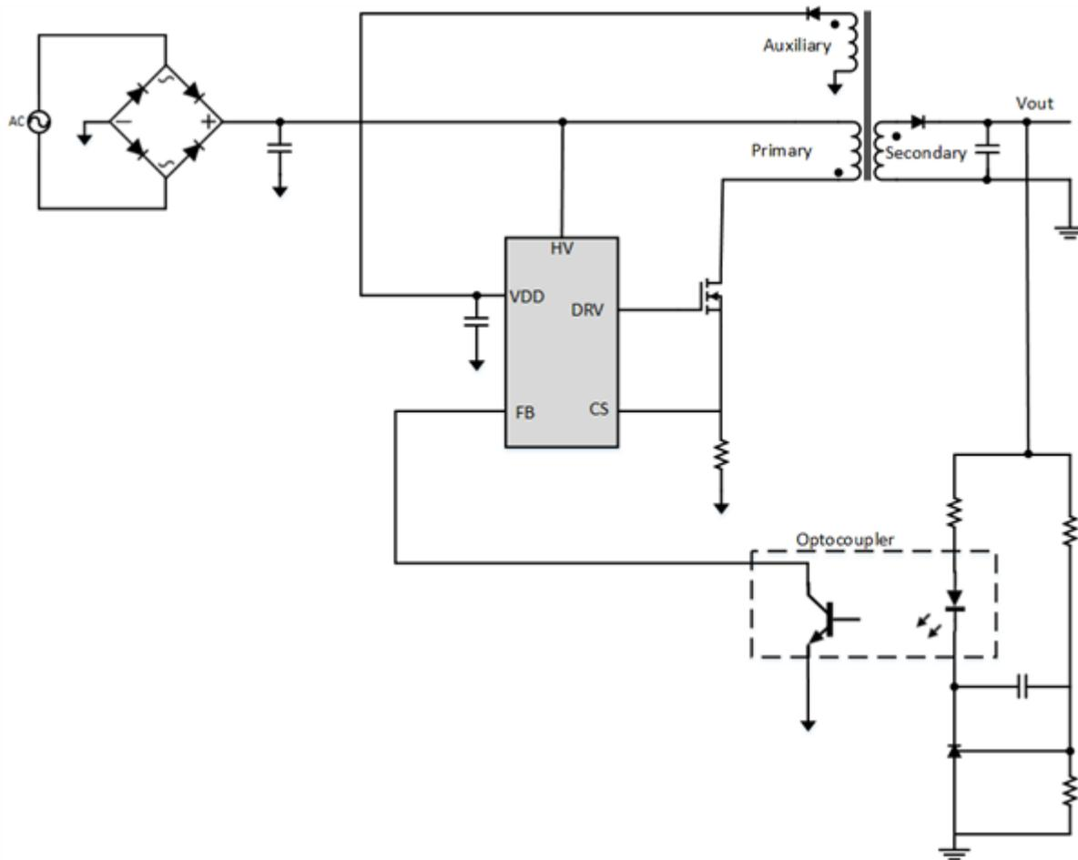
**Figure 3. AC/DC Flyback with Secondary-side Regulation Using Optocoupler Feedback**
