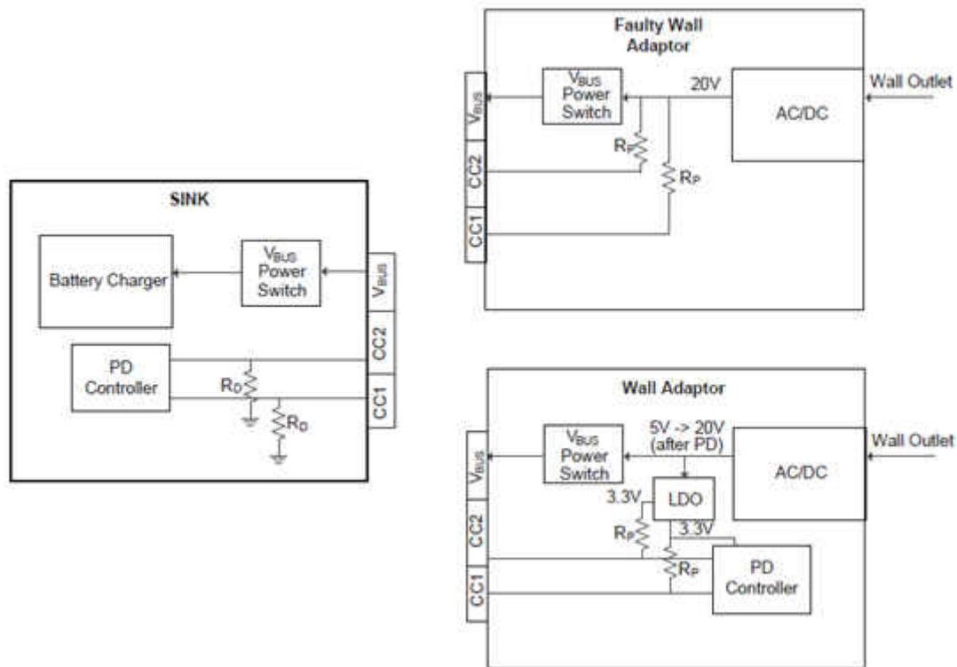
**Figure 2. CC Pin Exposure for Regular and Faulty Wall Adapters**
