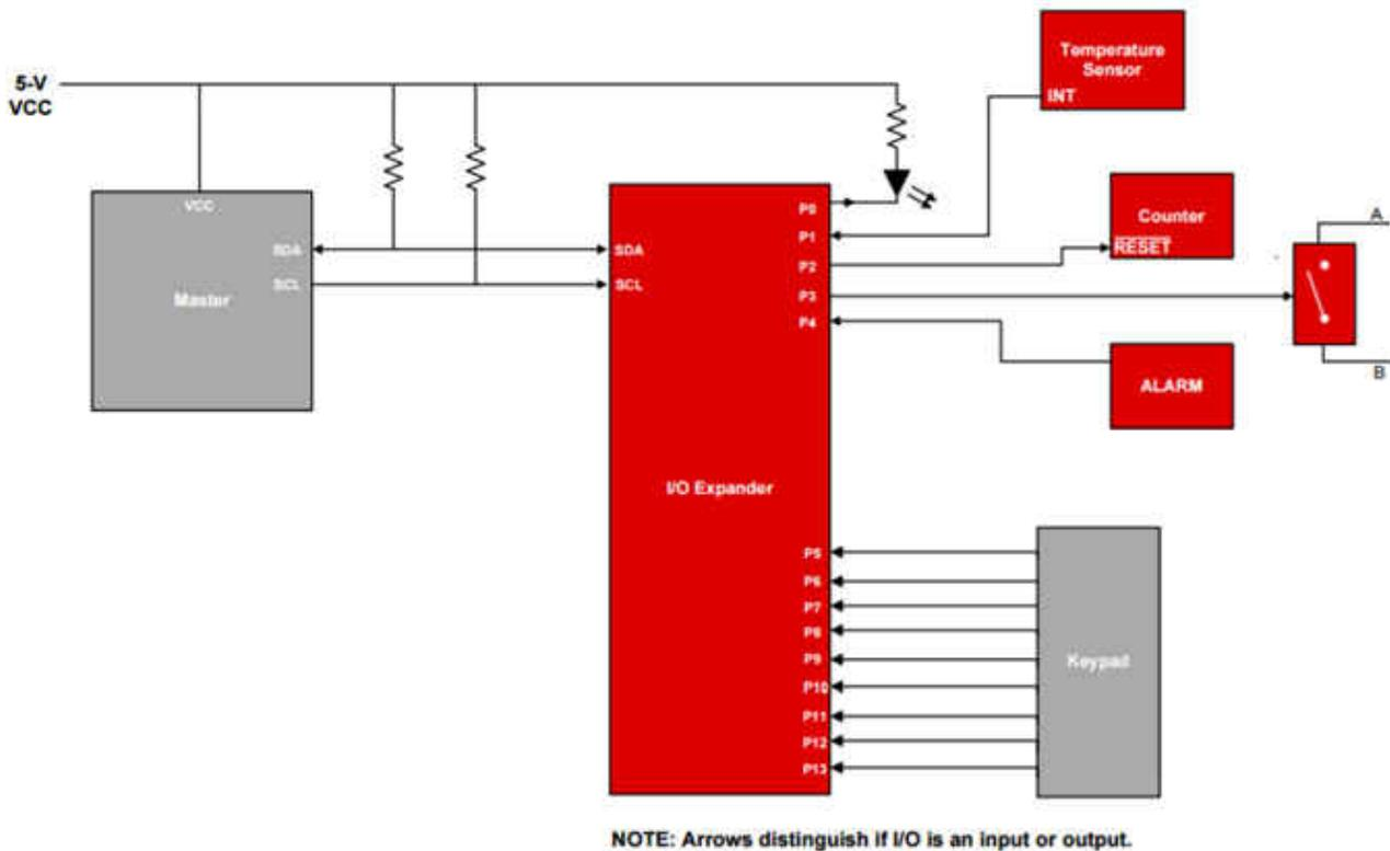
**Figure 2. A Microcontroller or Processor Using an I/O Expander to Control Peripherals**
