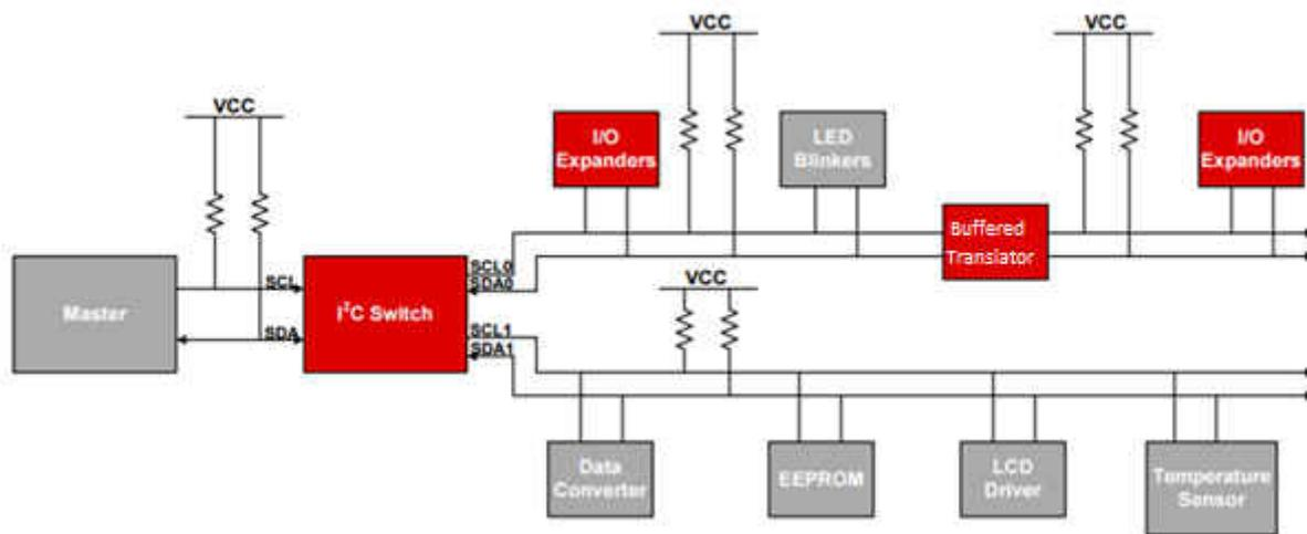
**Figure 1. An Electronic System with Various I<sup>2</sup>C Functional Devices**
