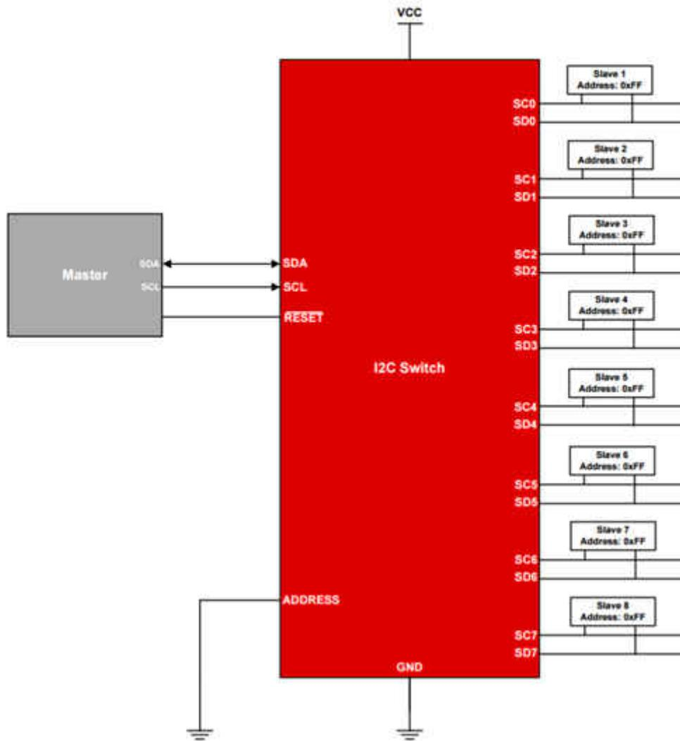
Figure 3. I<sup>2</sup>C Switch Example with Eight Channels
