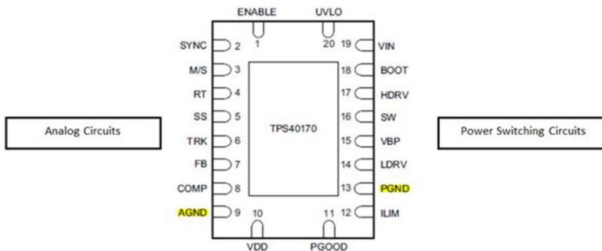
**Figure 7. Buck Controller IC Pinout for Analog and Power Connections**
