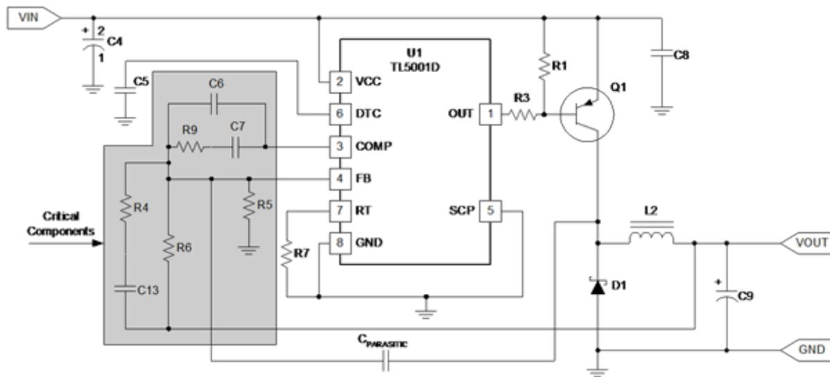
Figure 3. Feedback compensation network placement
