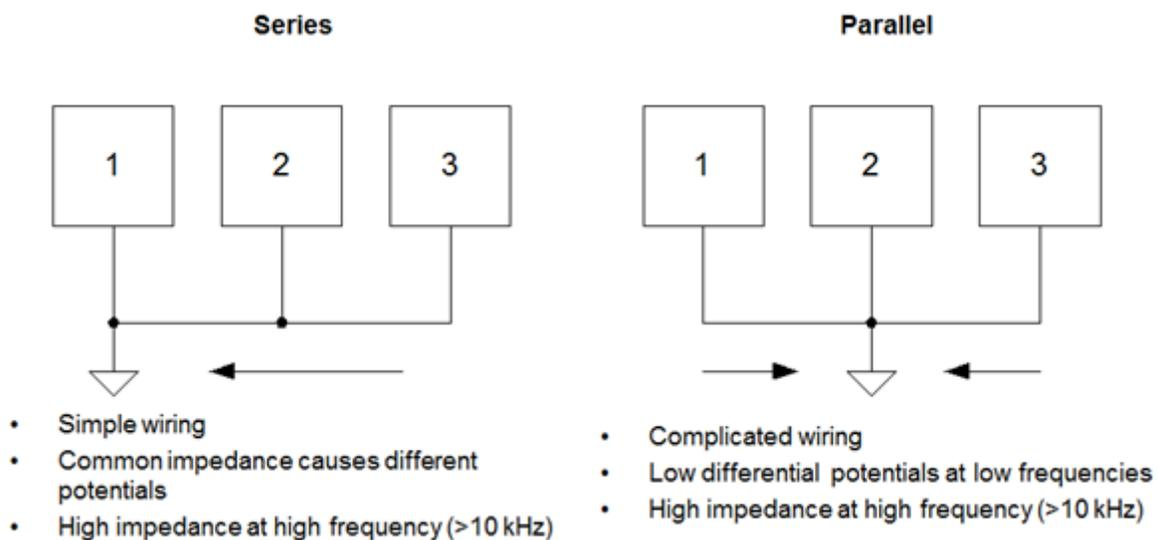
**Figure 5. Series and Parallel Single-point Ground Connections**
