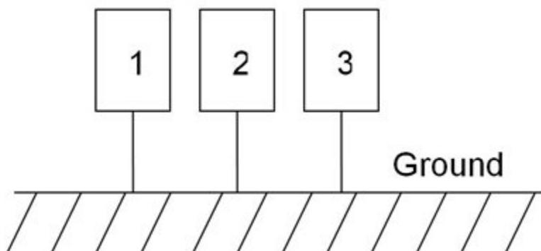
**Figure 6. Multipoint Ground Connections**
