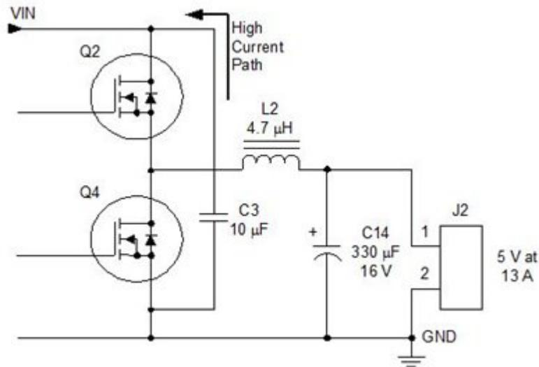
**Figure 4. Power Component Connections Indicating a High-current Path**
