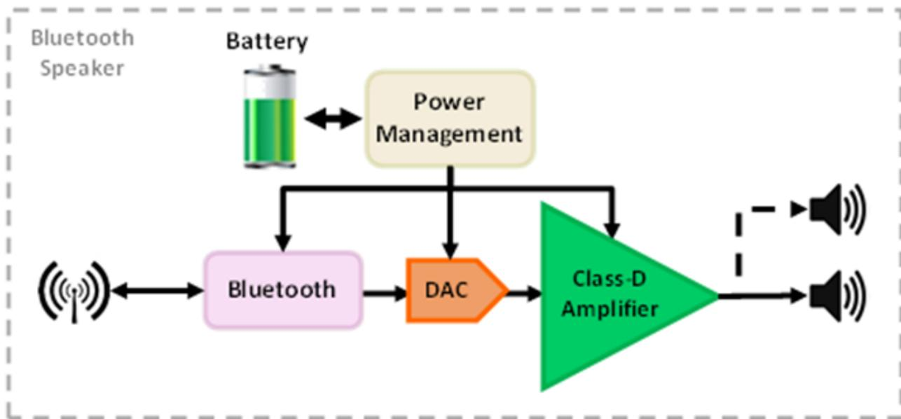
**Figure 1. Bluetooth Speaker Block Diagram**
