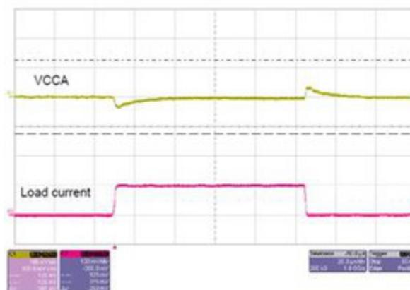
Figure 1. VCCA Transient Response to a 50% Load Step
