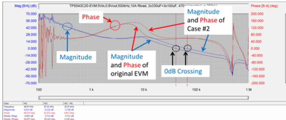
Figure 2. Bode Plot Comparison between Original Configurations versus Case No. 2
