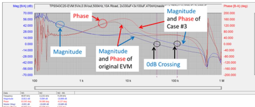
Figure 3. Bode Plot Comparison between Original Configurations versus Case No. 3
