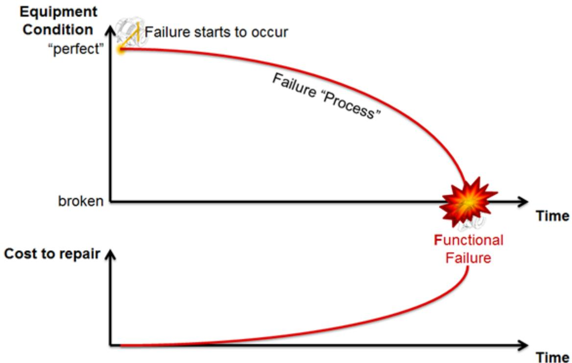
Figure 1. Failure Process and Cost to Repair
