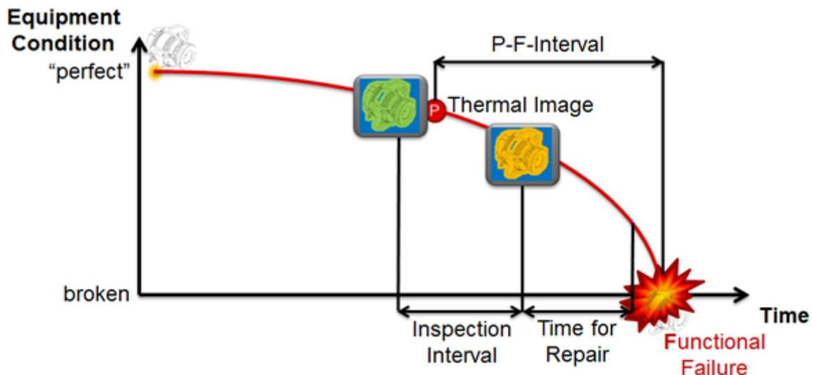
Figure 3. Inspection Interval
