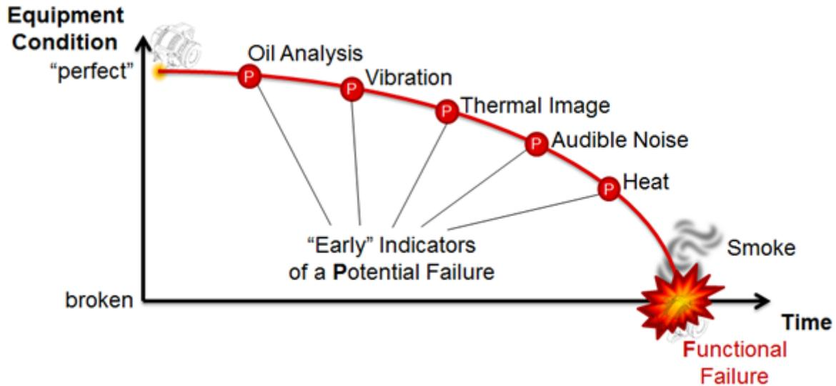
Figure 2. P-F Curve – Potential Failure to Functional Failure
