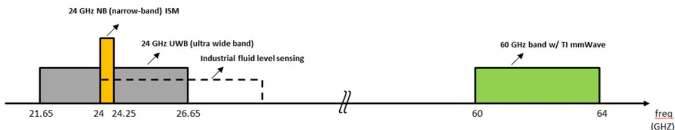
**Figure 1. Comparison between the 24-GHz Narrowband and 60-GHz Ultrawide Frequency Bands**
