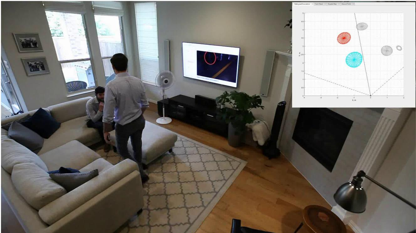
**Figure 2. Using 60-GHz mmWave Sensors for People Classification (Red and Blue) and False Detection Mitigation (Gray)**
