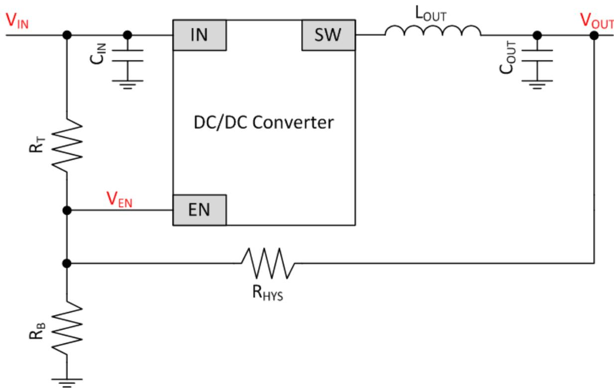
Figure 1. Simplified DC/DC Converter Schematic
