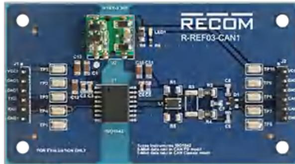
Figure 3. Isolated Power Using Power Modules
