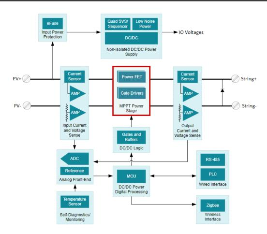
The solar power optimizer shows the job of the MOSFET, which is to condition the voltage from the solar panel's photovoltaic cells (PV+/PV-) before sending it to a central inverter (String+/String-) to finish the DC/AC conversion. These MOSFETs need to be able to reach high voltages during DC/DC conversions and thus need a gate driver because the FETs cannot be driven directly by a microcontroller.
