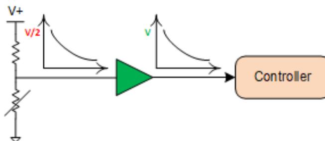
**Figure 3. NTC Thermistor Sensing Circuit**
