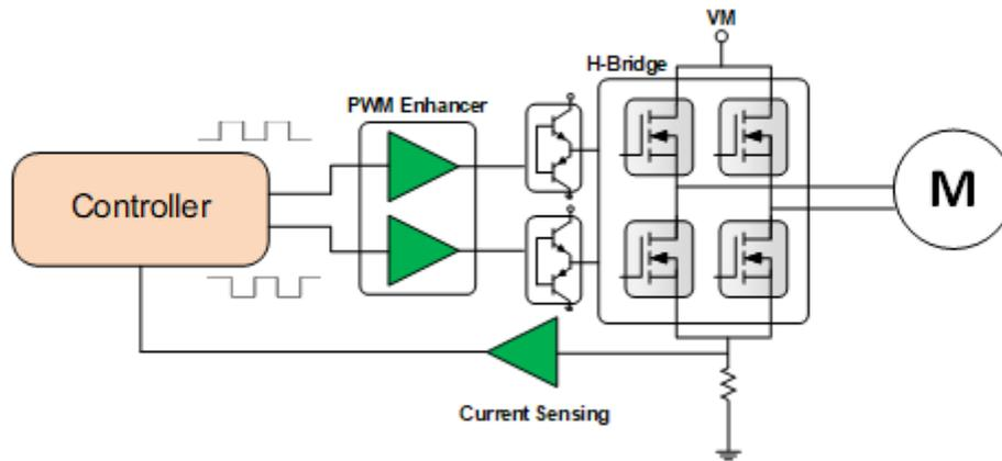
**Figure 5. Enhanced PWM Circuit**
