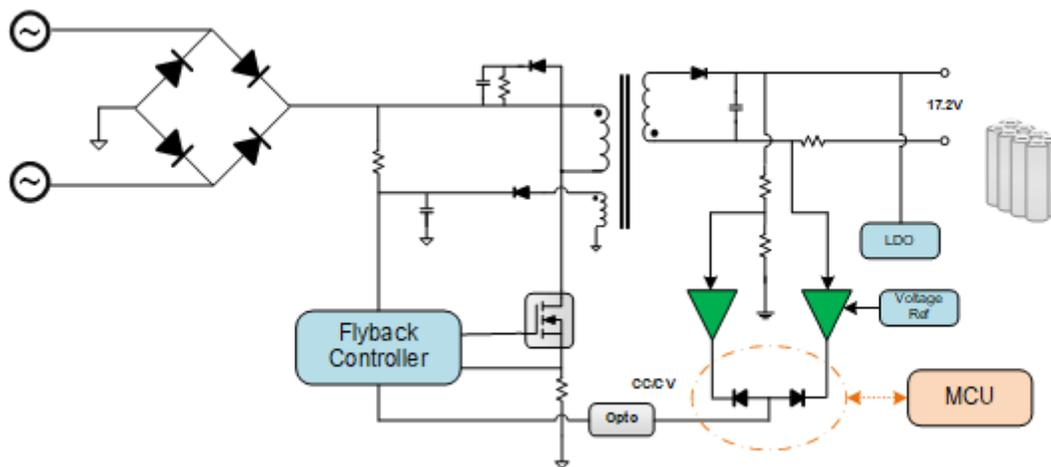
**Figure 2. A Discrete Battery Charger Circuit**
