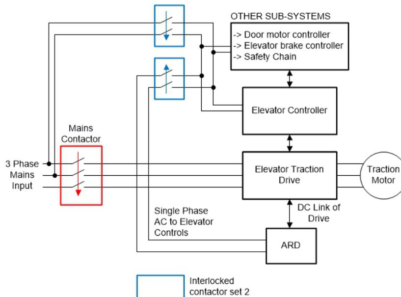
**Figure 3. An ARD system with a bidirectional DC/DC converter connected into an elevator system**
