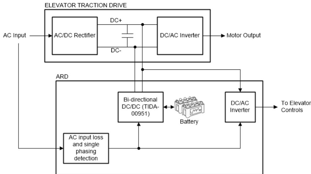
**Figure 4. An ARD with a bidirectional DC/DC**
