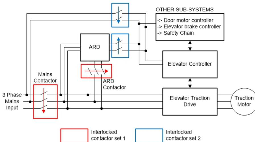
Figure 1. Conventional ARD system connection in an elevator
