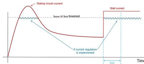
**Figure 3. Typical brushed-DC motor profile for systems with possible stall events**
