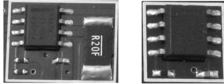
Figure 1. The DRV8870 with an external shunt resistor vs. the DRV8871 with integrated current sensing
