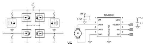
**Figure 4. Discrete H-bridge circuit (a); integrated motor driver H-bridge with the DRV8837C (b)**
