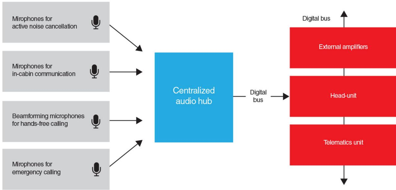
**Figure 4. A centralized audio hub module**
