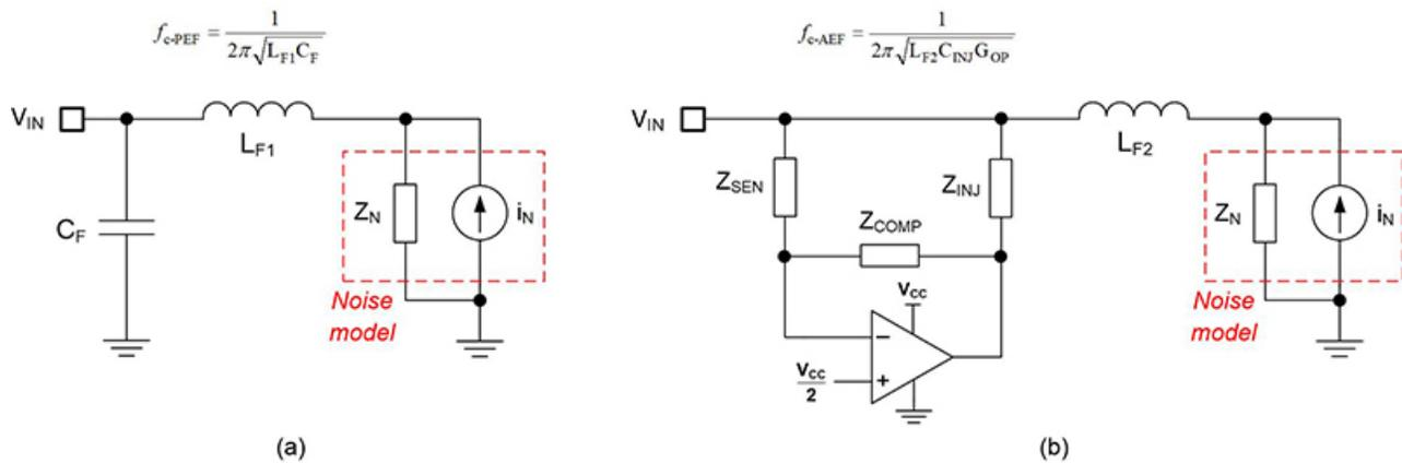
**Figure 1. Conventional passive filtering (a) and active filtering (b) circuit implementations**
