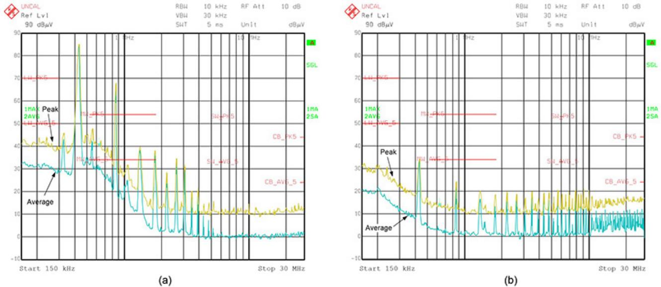
**Figure 3. Comparing filtering performance when AEF is disabled (a) and enabled (b)**
