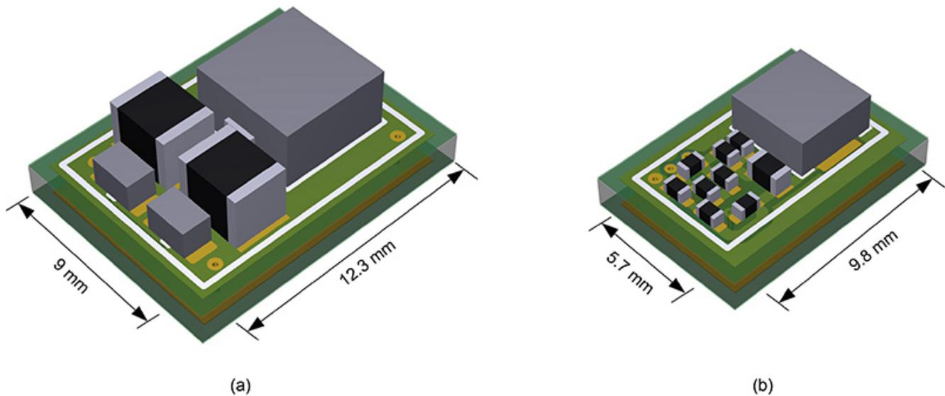
**Figure 4. PCB layout size comparison of passive (a) and active (b) filter designs**
