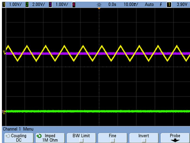
**Figure 7. LM393 Cold Temperature Performance outside  $V_{CM}$**
