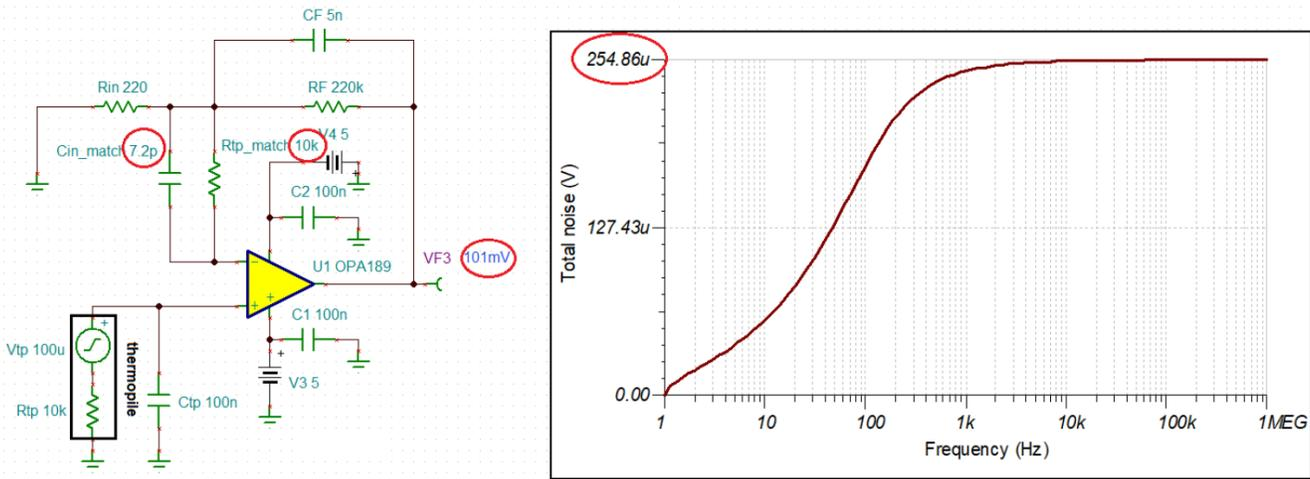
**Figure 3. The OPA189 in a Thermopile Application with Matching Input Impedance**
