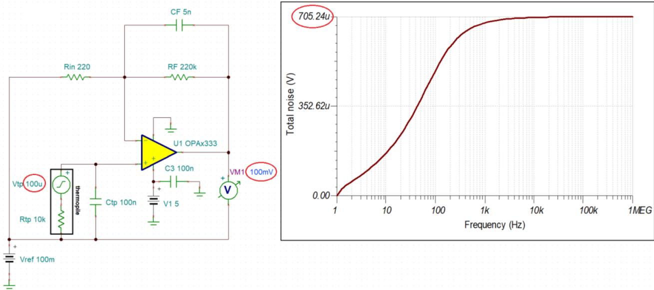
**Figure 1. The OPA333 in a Thermopile Application with G = 1,001**
