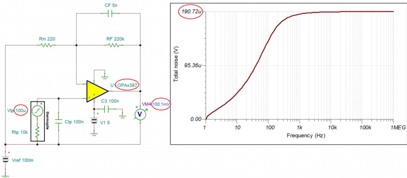
**Figure 4. The OPA387 in a Thermopile Application with G = 1,001**
