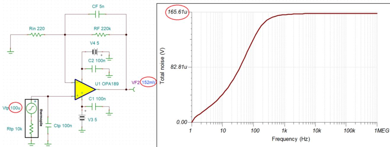
**Figure 2. The OPA189 in a Thermopile Application with G = 1,001**
