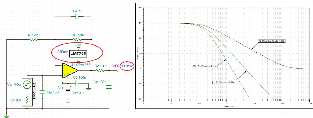
**Figure 6. The OPA387 Thermopile Application with the LM7705 Negative Charge Pump and Output Filtering**
