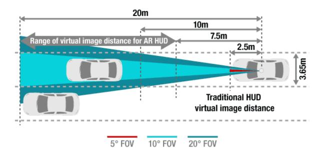
Figure 1. The Range of AR HUD Image Distance with DLP Technology.
