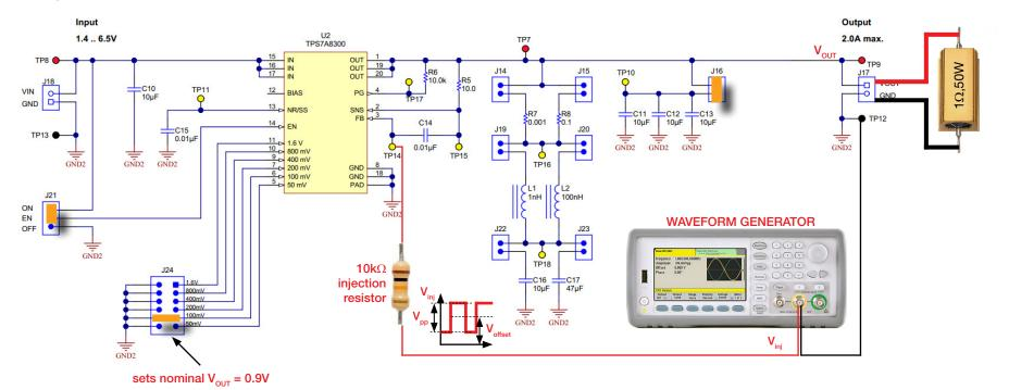
Figure 13. TPS7A8300 board operating as dynamic load
