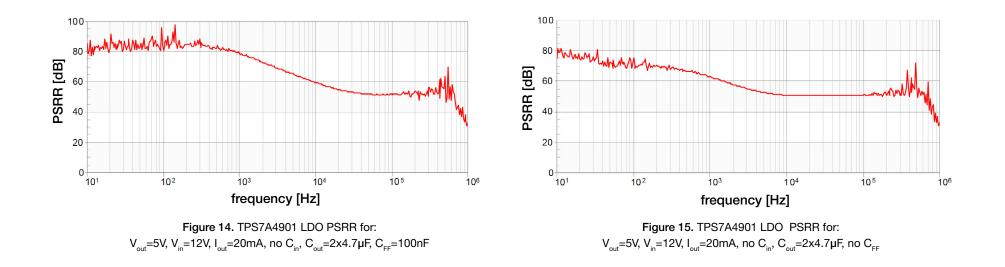
The plots of Figures 14 and 15 highlight the expected influence of the phase lead capacitance on the TPS7A4901 LDO regulator closed-loop PSRR. In Figure 14 you can observe a higher PSRR, compared to the plot of Figure 15, in the middle-to-high frequency region, where the zero introduced by the phase lead capacitance has a strong effect on the increase of the crossover frequency, thus improving the PSRR.
