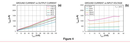
The LDO regulator sinks a quiescent current I<sub>o</sub> from the line, even when it is not delivering current to the load (see [1][2][12] for details).
