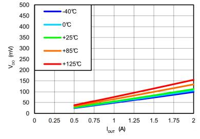
Figure 8. TPS7A8300 LDO regulator droupout voltage vs output current for: V\_{out}=0.8V and V\_{in}=1.4V
