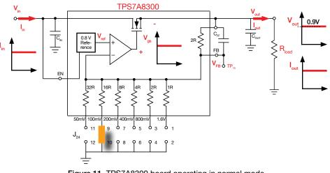
Figure 11. TPS7A8300 board operating in normal mode
