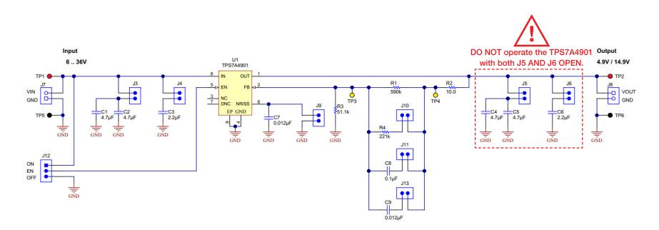
Figure 1. Circuit schematic of TI-PMLK TPS7A4901 LDO regulator
