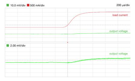
Figure 18. TPS7A8300 LDO regulator load transient response for:  $V_{in}$ = 1.8V,  $V_{out}$ =1.5V,  $I_{out}$ =0.1A $\rightarrow$ 0.9A,  $C_{out}$ =C<sub>16</sub>=10µF,  $L_{out}$ =L<sub>1</sub>=1nH, ESR<sub>out</sub>=R<sub>7</sub>=1mΩ
