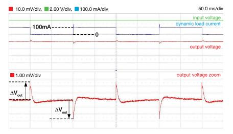
Figure 16. TPS7A4901 LDO load transient for:  $V_{out}$ =5V,  $V_{in}$ =6V,  $C_{out}$ =11.6µF,  $C_{FF}$ =12nF and  $I_{OUT}$  swinging between 50mA and 150mA
