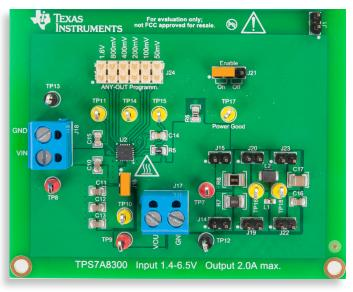
Figure 6. TPS7A8300 LDO board: jumpers set-up for Test#1
