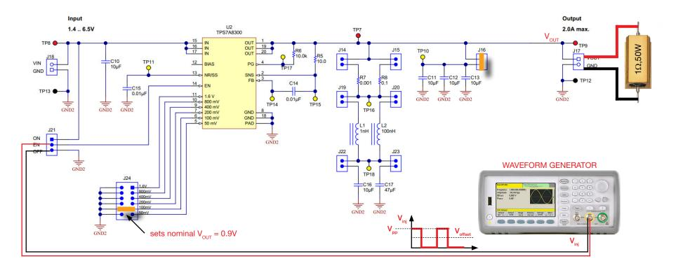
Figure 8. TPS7A8300 board operating as dynamic load
