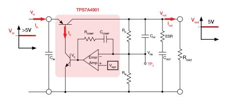
Figure 6. TPS7A4901 board operating in normal mode
