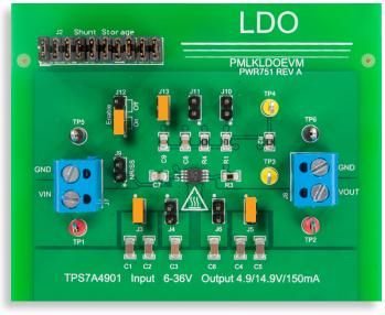
Figure 7. TPS7A4901 LDO board: jumpers set-up for Test#2
