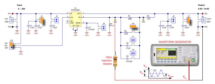
Figure 8. TPS7A4901board operating as dynamic source
