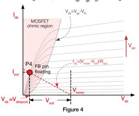
In the ohmic region, the MOSFET drain-source current  $I_{ds}$  is given by equation (4):
