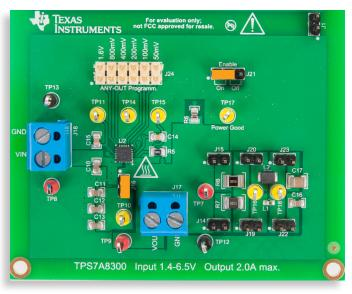
Figure 7. TPS7A8300 LDO board: jumpers set-up for Test#2
