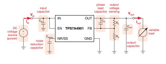
Figure 1. Simplified schematic of the TPS7A4901 LDO regulator
