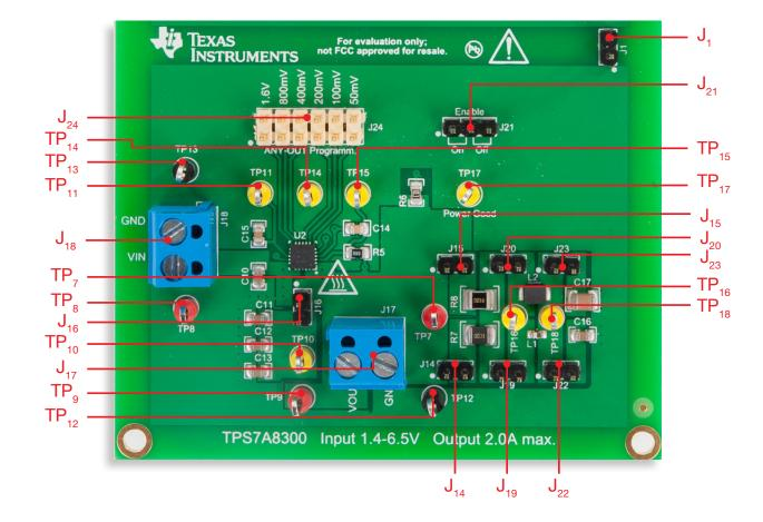
Figure 4. Plain view of TI-PMLK TPS7A8300 LDO regulator board
