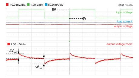
Figure 18. TPS7A4901 LDO line transient for V\_{\_{out}}=5V, I\_{\_{OUT}}=50mA, C\_{\_{FF}}=12nF and V\_ $_{\rm IN}$  switching between 6V and 8V
