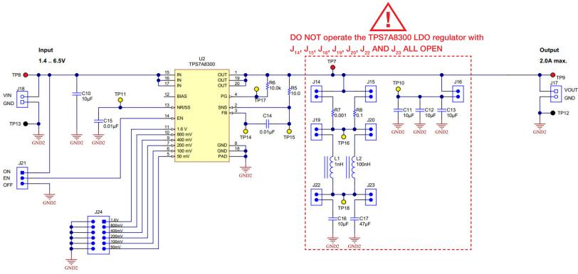
Figure 3. Circuit schematic of TI-PMLK TPS7A8300 LDO regulator
