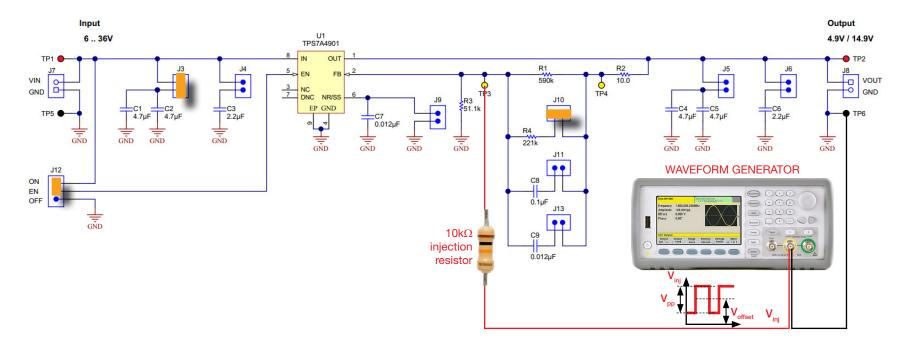
Figure 13. TPS7A4901 LDO REGULATOR operating as dynamic source
