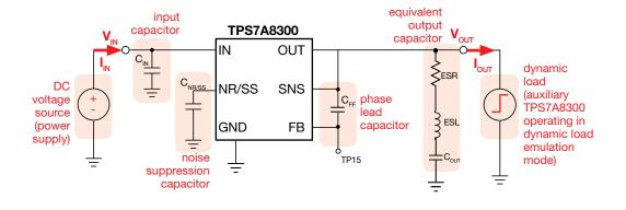
Figure 1. Simplified schematic of the TPS7A8300 LDO regulator
