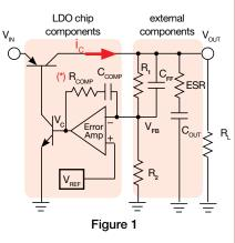
(\*) The resistor  $\mathbf{R}_{\text{COMP}}$  is typically used in LDOs designed to work with ceramic output capacitors.
