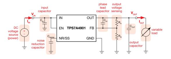
Figure 1. Simplified schematic of the TPS7A4901 LDO regulator
