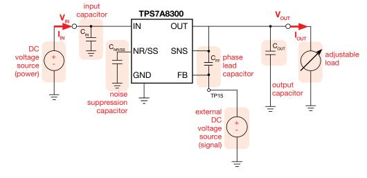
Figure 1. Simplified schematic of the TPS7A8300 LDO regulator
