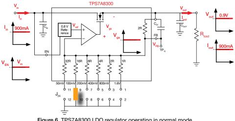
Figure 6. TPS7A8300 LDO regulator operating in normal mode
