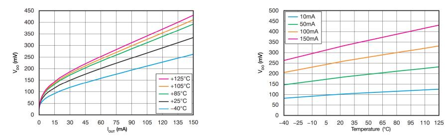
Figure 8. Dropout voltage of TPS7A4901 vs load current
