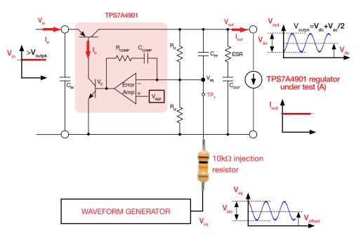
Figure 7. TPS7A4901 board operating in dynamic source emulation mode
