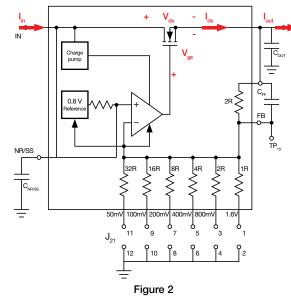
The output voltage is regulated if the MOSFET operates in the saturation region, where  $V_{ds}$ - $V_{th}$ , as in Figure 3.
