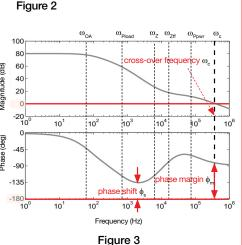
The  $\rm G_{\rm VC}$  and  $\rm G_{\rm EA}$  gains depend on LDO chip internal components (pass device, gate driver, op-amp, error amplifier feedback  $\rm R_{\rm COMP}\text{-}C_{\rm COMP}$ ), on external R-C components ( $\rm R_{f1},\,\rm R_{f2},\,\rm C_{FF},\,\rm C_{\rm OUT},\,\rm ESR$ ) and on load current  $\rm I_{\rm OUT}.$  The resulting loop gain is given by equation (1):
