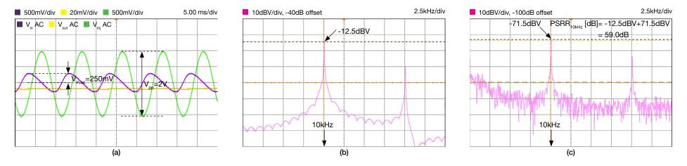
Figure 17. FFT-based PSRR measurement of TPS7A4901 regulator under test for  $f_{ac}=10$ kHz,  $V_{inj,offset}=1.19$ V,  $V_{inj,offset}=1.19$ V,  $V_{in,ac}=250$ mV,  $V_{out}=4.9$ V,  $I_{out}=50$ mA, no  $C_{in}$ ,  $C_{out}=2x4.7\mu$ F,  $C_{FF}=100$ nF: (a) time domain waveforms; (b)  $V_{in,ac}$  FFT magnitude plot; (c)  $V_{out,ac}$  FFT magnitude plot.
