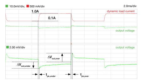
**Figure 15.** TPS7A8300 LDO regulator load transient response for:  $V_{in}$ = 1.8V,  $V_{out}$ =1.5V,  $I_{out}$ =0.1A $\leftrightarrow$ 1.0A,  $C_{out}$ =C<sub>16</sub>=10µF,  $L_{out}$ =L<sub>2</sub>=100nH, ESR<sub>out</sub>=R<sub>8</sub>=100mΩ
