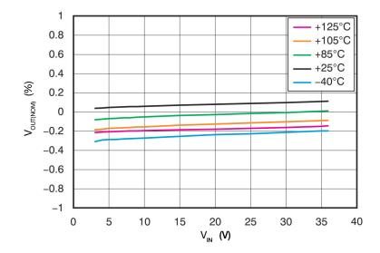
Figure 10. Line regulation of TPS7A4901, with temperature dependency
