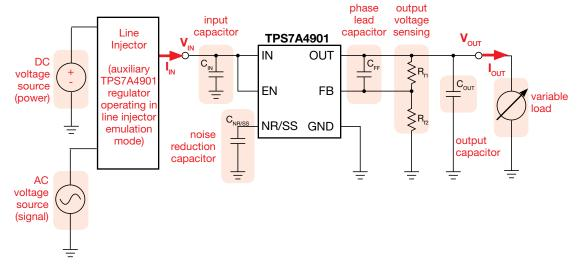
Figure 1. Simplified schematic of the TPS7A4901 LDO regulator
