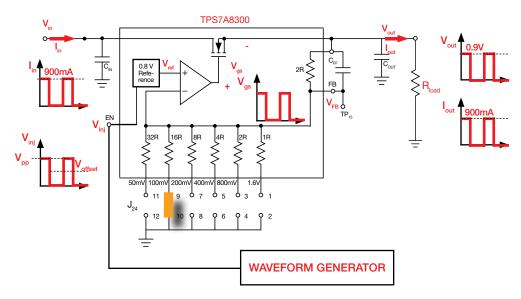
Figure 7. TPS7A8300 LDO regulator operating in dynamic load emulation mode
