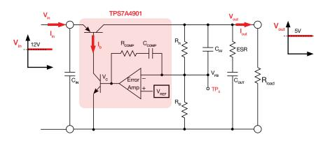
Figure 11. TPS7A4901 LDO regulator operating in normal mode
