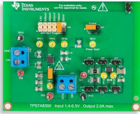
(b) TPS7A8300 LDO regulator operating as dynamic load Figure 14. Jumpers set-up for Test#2
