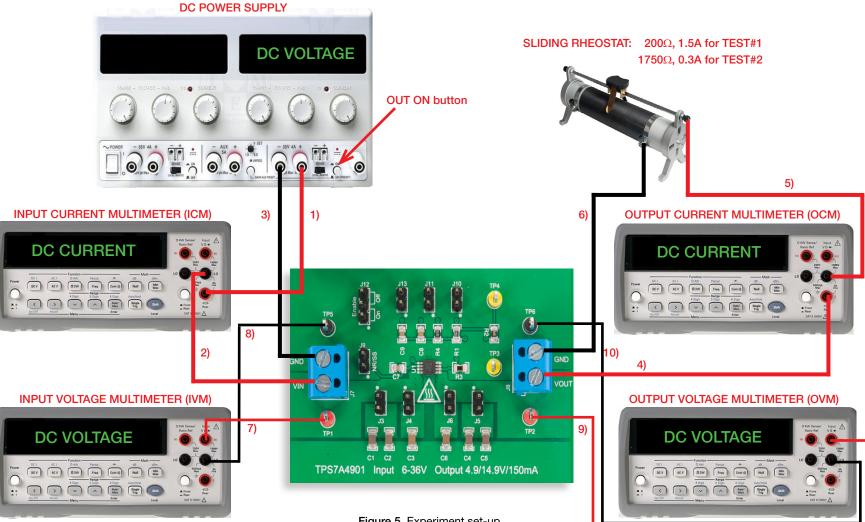
Figure 5. Experiment set-up.
