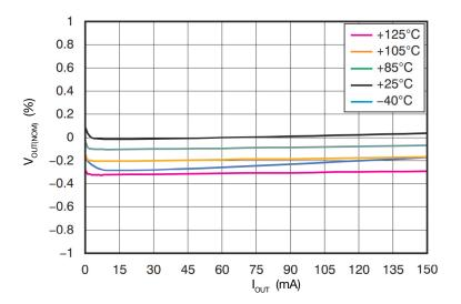
Figure 11. Load regulation of TPS7A4901, with temperature dependency
