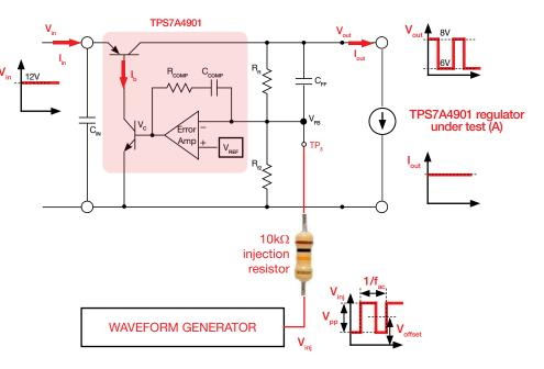
Figure 12. TPS7A4901 LDO regulator operating in dynamic source emulation mode
