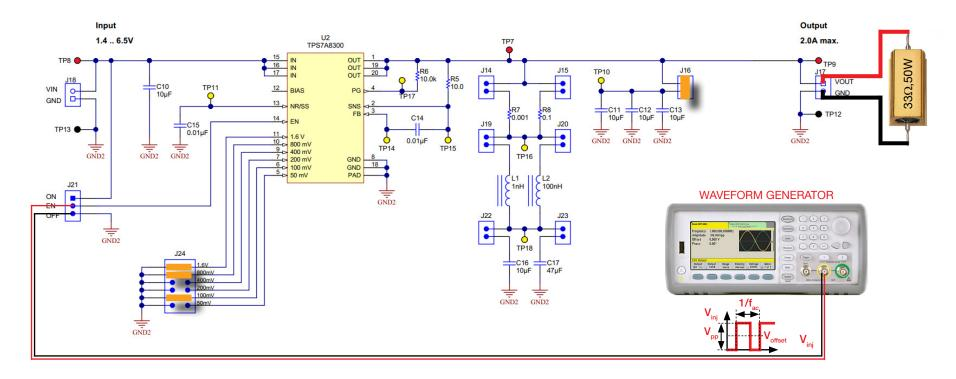
Figure 8. TPS54160 board operating as dynamic load
