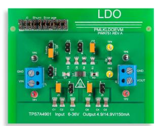
(b) TPS7A4901 LDO regulator operating as line injector
