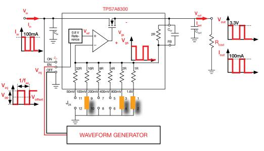
Figure 7. TPS7A8300 board operating in dynamic load emulation mode
