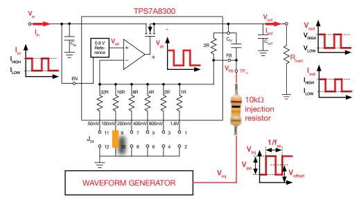
Figure 12. TPS7A8300 board operating in dynamic load emulation mode
