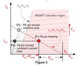
In the saturation region, the MOSFET drain-source current  ${\rm I}_{\rm rs}$  is given by equation (3):
