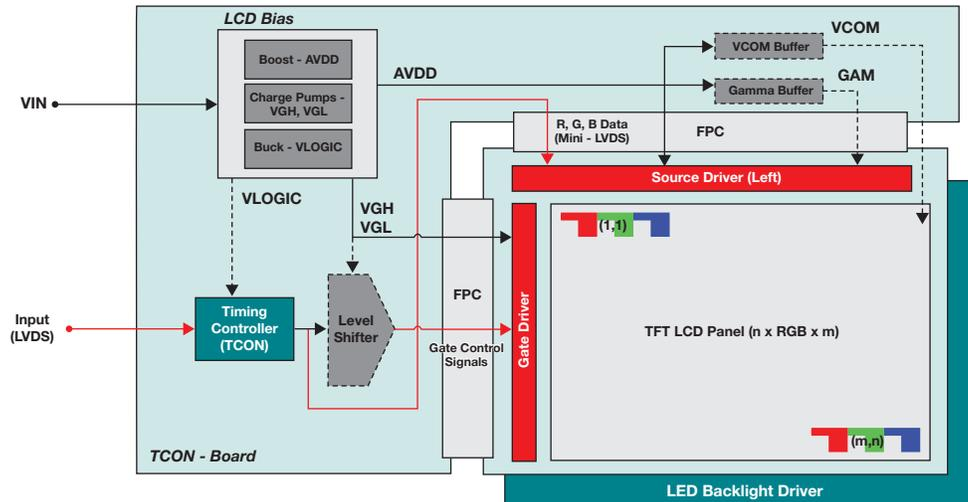
Figure 2. Block diagram of a TFT LCD subsystem.
