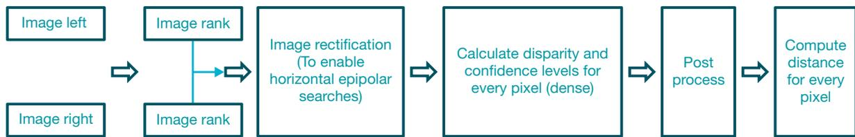
Figure 9: A high-level data and algorithm flow for stereo disparity-based distance computation.
