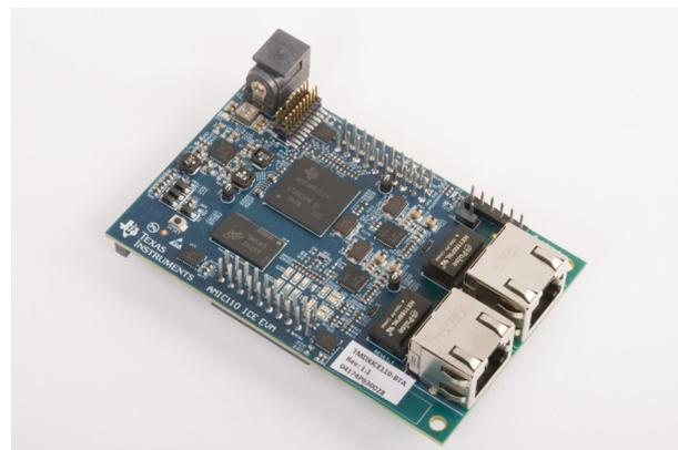
Figure 5. AMIC110 Industrial Communications Engine (ICE).
