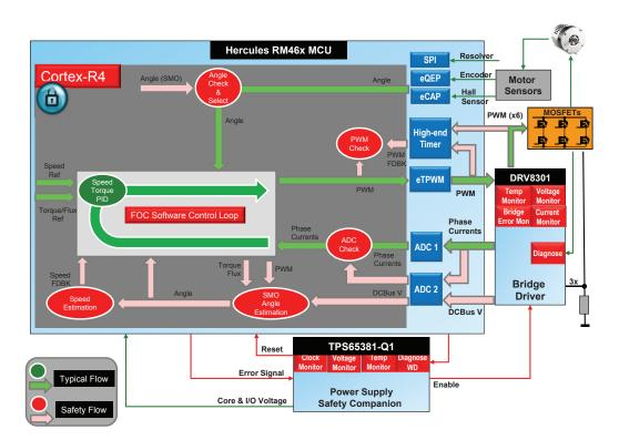
Figure 1. Motor control system block diagram with safety checks.
