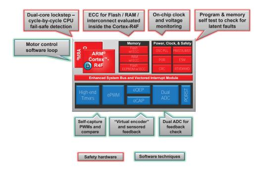
Figure 2. Block diagram of TI safety microcontrollers with hardware safety features.
