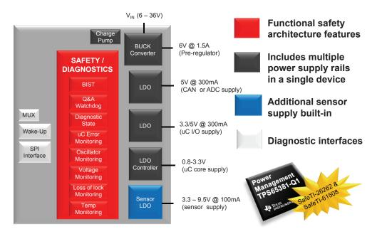
Figure 7. The TPS65381-Q1 multi-rail safety PMIC
