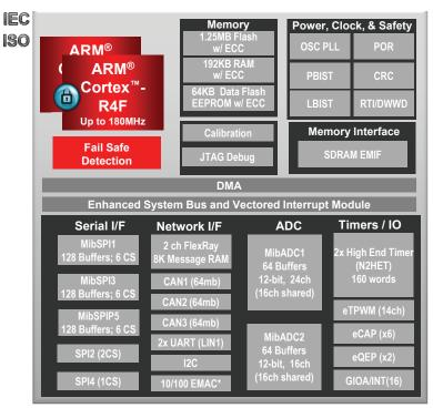
Packages: LQFP: 144pin -20x20; nfBGA: 337 pin-16x16, 0.8mm; -40 to 125 C Temperature Range
