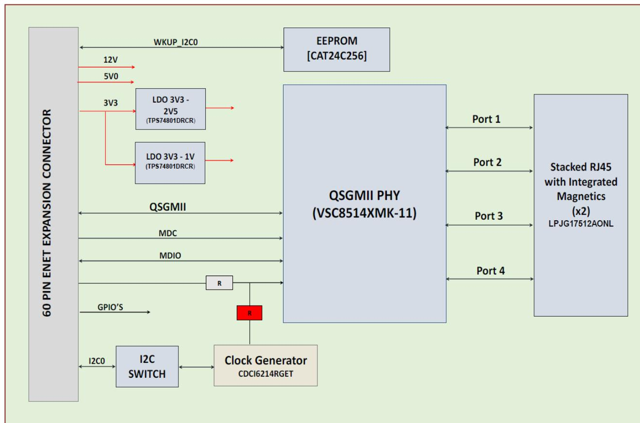
Figure 3-1. Functional Block Diagram of QP-ENET Expansion Board
