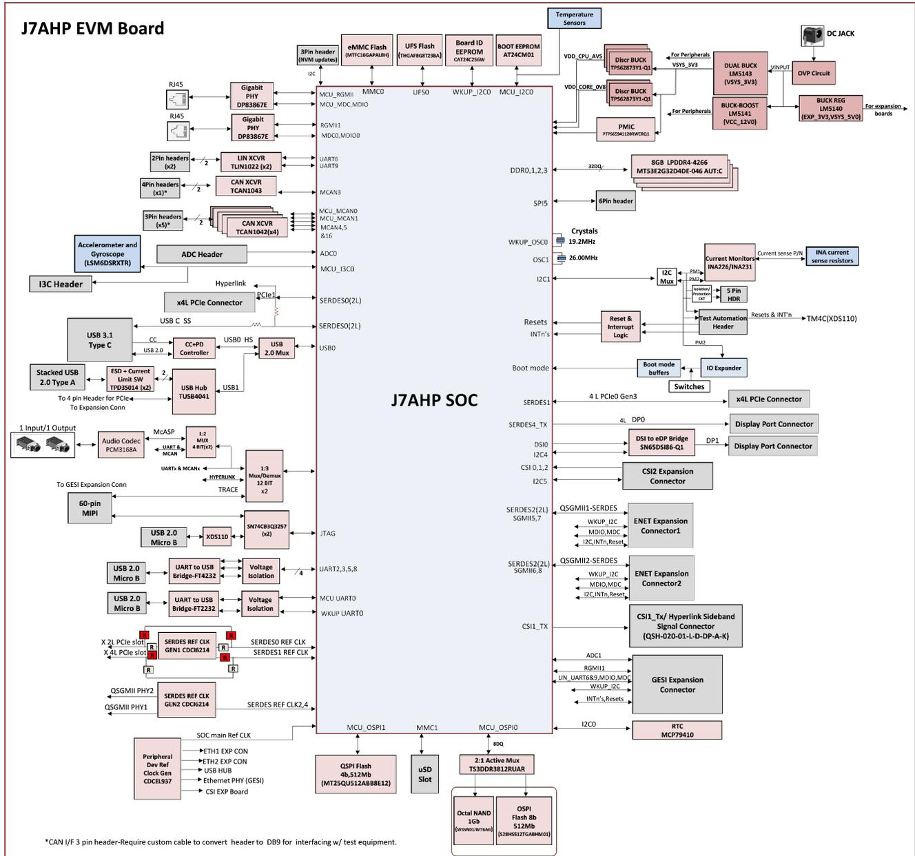
Figure 3-1. J7AHP EVM Board Functional Block Diagram
