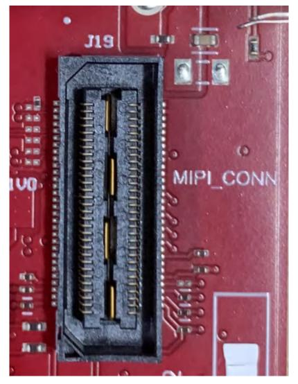
Figure 2-8. 60-pin MIPI Connector
