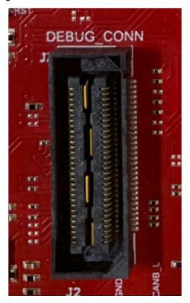
Figure 2-9. 60-pin Debug Connector
