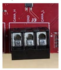
Figure 2-10. CAN\_A Connector
