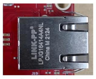
Figure 2-12. RJ45 Connector
