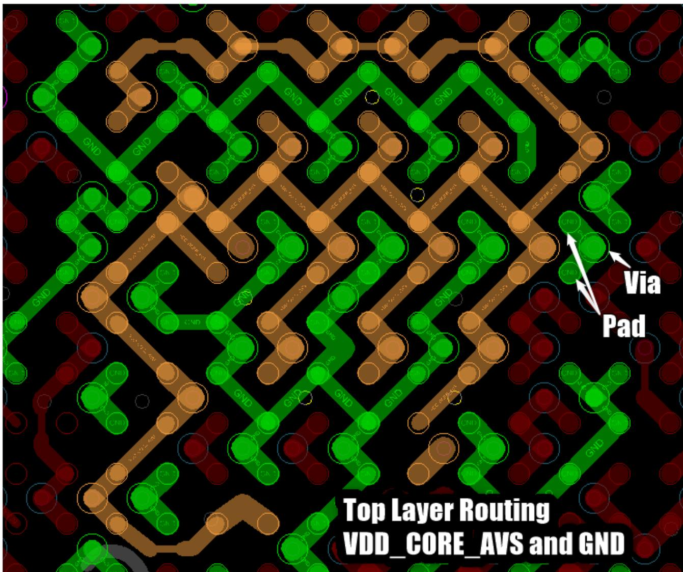
Figure 15. Via Sharing on the Top Layer
