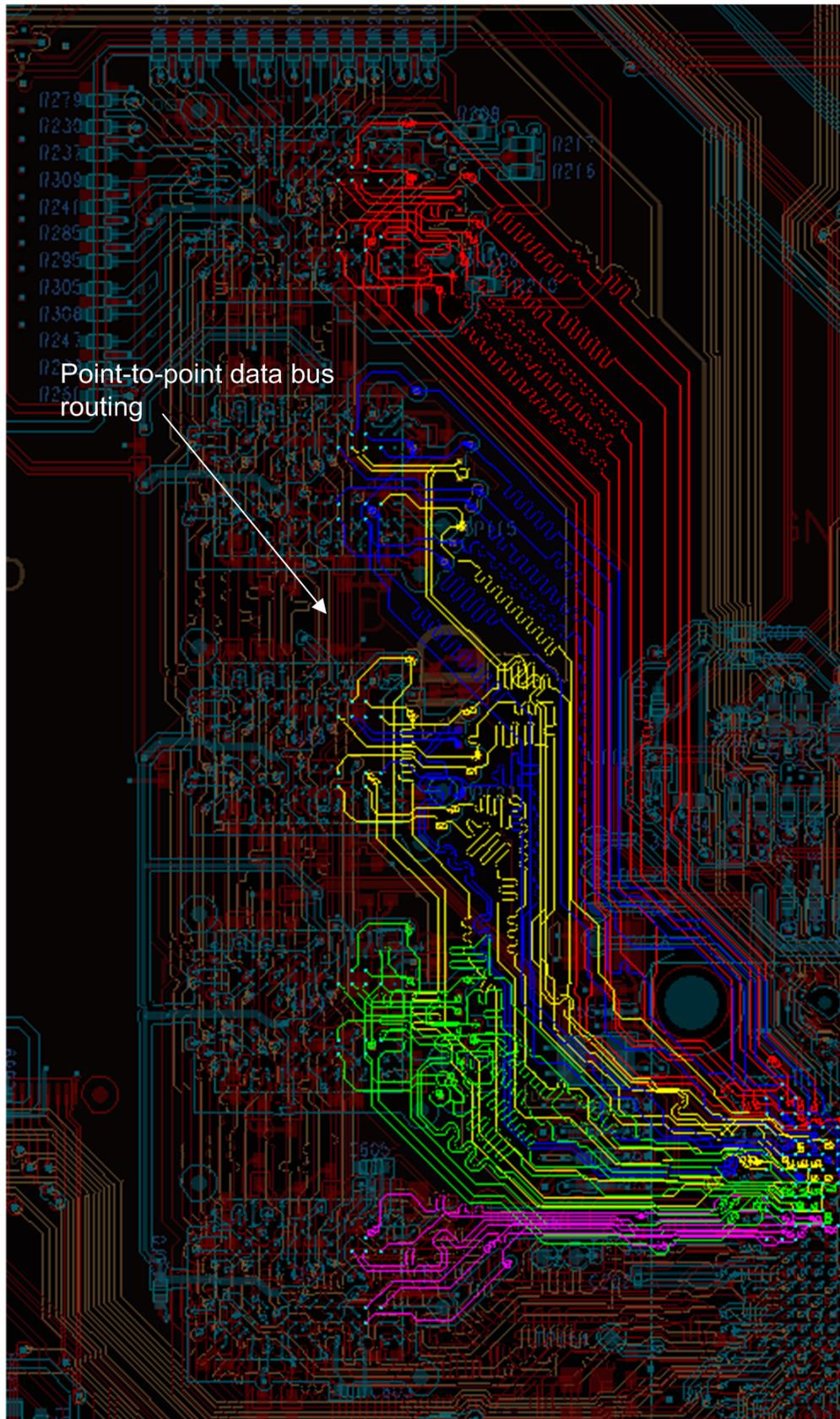
Figure 1-3. DDR3 Data Group Routing
