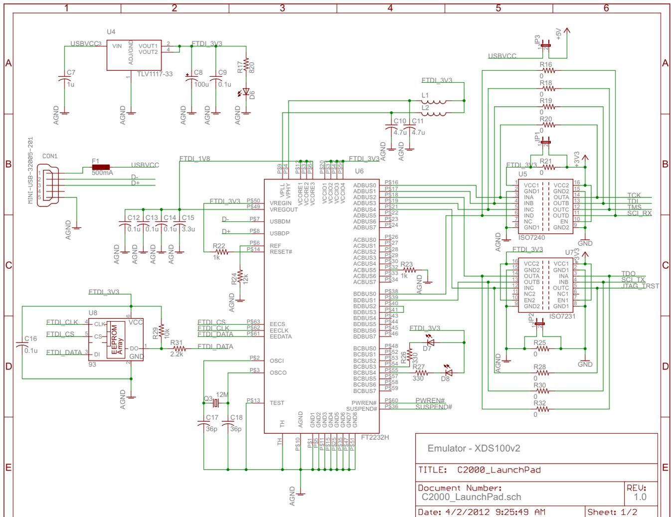
Figure 2. C2000 LaunchPad Schematic—Sheet 1 of 2
