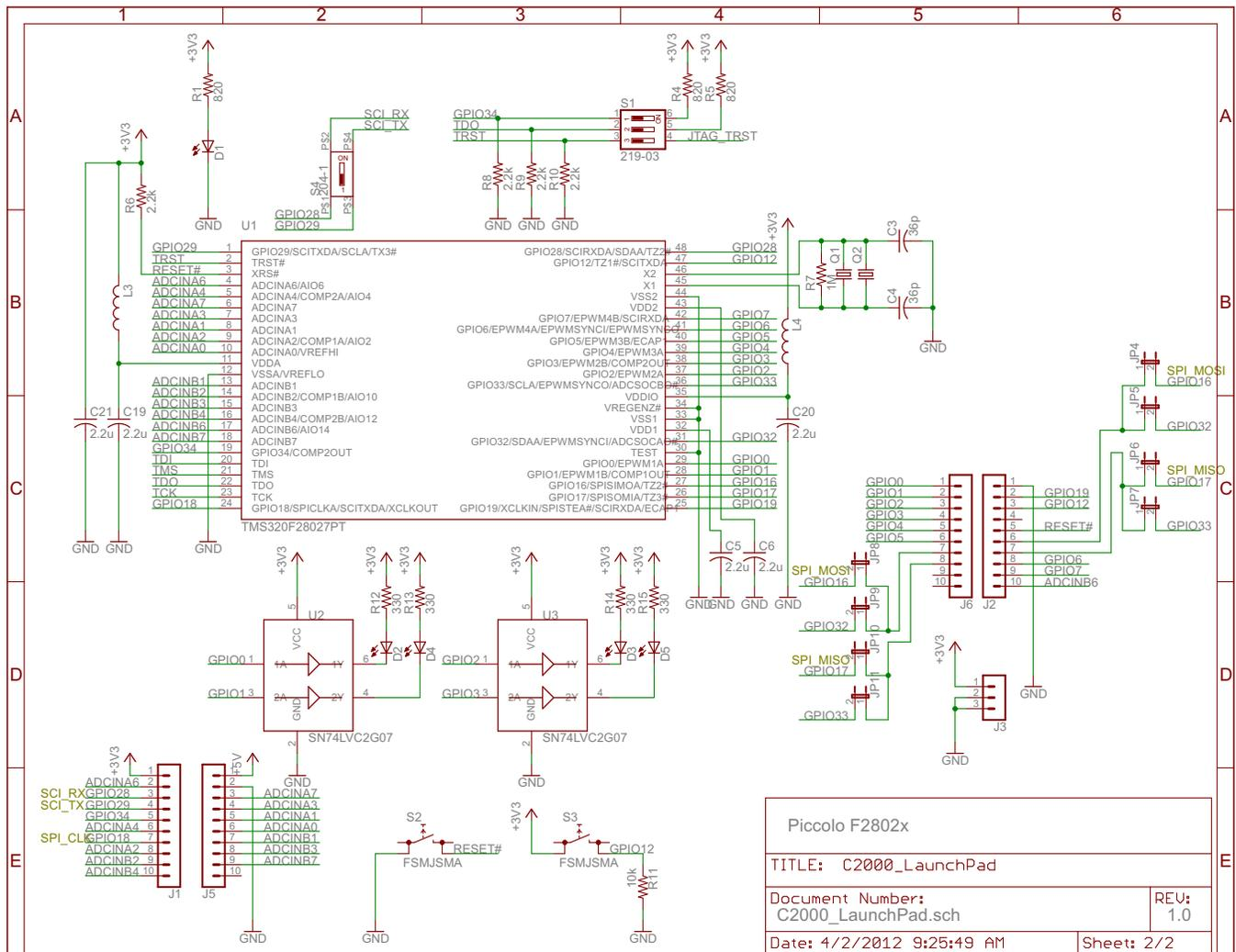
Figure 3. C2000 LaunchPad Schematic—Sheet 2 of 2
