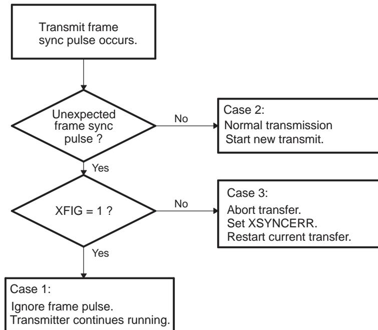
**Figure 31. Unexpected Transmit Frame Synchronization Pulse**
