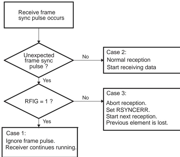
**Figure 26. Unexpected Receive Frame Synchronization Pulse**
