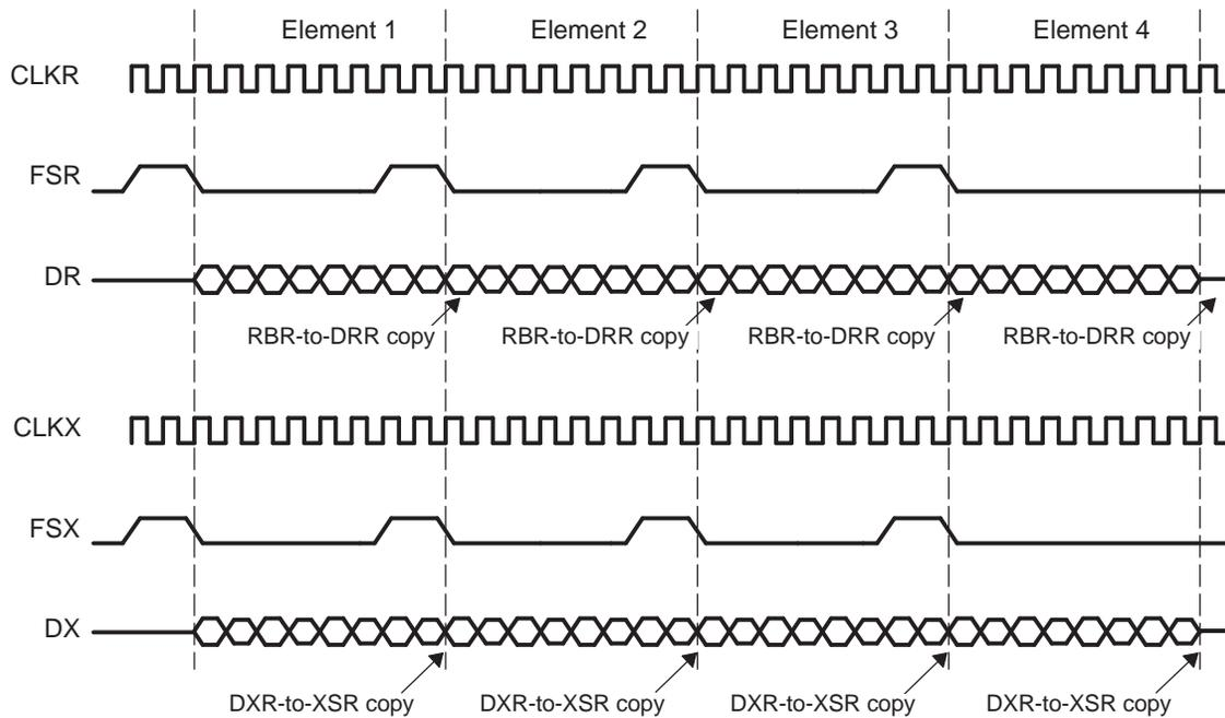
**Figure 22. Data Packing at Maximum Frame Frequency With (R/X)FIG = 1**
