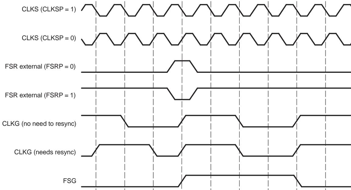
When GSYNC = 1, the transmitter can operate synchronously with the receiver, provided that the following conditions are met:
