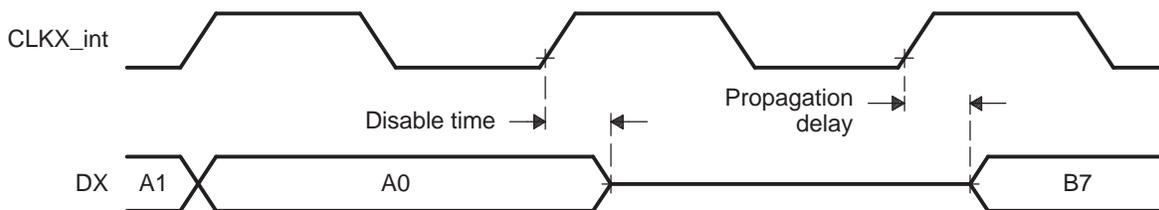
**Figure 4. Receive Data Clocking**
