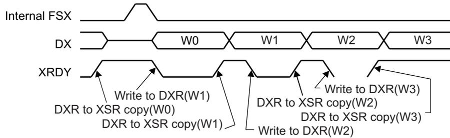
(b)  $XMCM = 1h$ ,  $XPABLK = 0$ ,  $XCERE0 = 0000\ 000Ah$ : Only channels 1 and 3 enabled and unmasked
