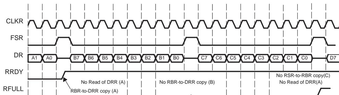
Figure 24. Serial Port Receive Overrun Avoided
