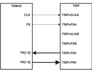
Figure 11. TSIP Connected to TEMUX
