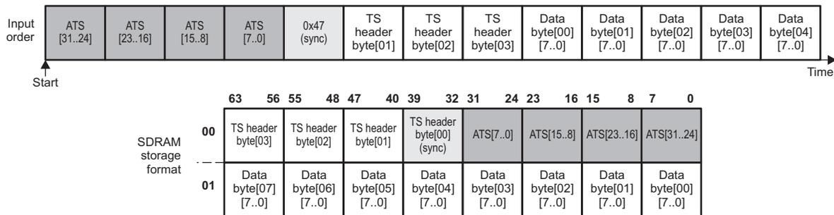
Figure 10. Bit-Level Endian Format in SDRAM Format
