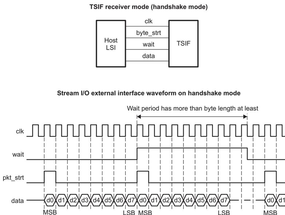
In transmitter mode, the wait signal from the external host device is detected by the TSIF module. The wait signal is latched by the pulse signal that indicates the start of a byte data (byte\_start signal for internal use). If the signal is detected by the TSIF module, the module stalls the output after a byte transfer is finished. The minimum unit of data transfer is a byte. All data with a data\_enable signal is detected by the external host device.
