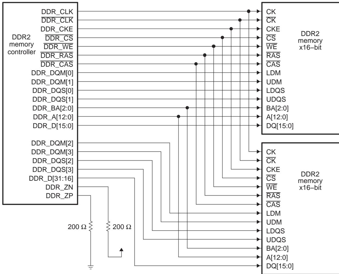
Figure 18. Connecting DDR2 Memory Controller for 16-Bit Connection
