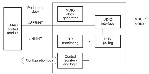
Figure 12. MDIO Module Block Diagram
