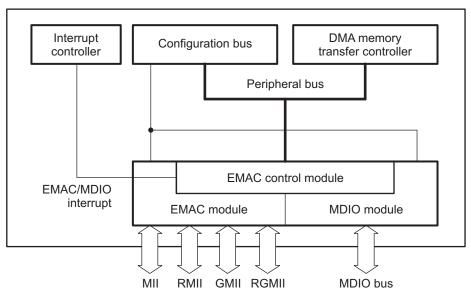
The EMAC control module is the main interface between the device core processor and the EMAC module and MDIO module. The EMAC control module contains the necessary components to allow the EMAC to make efficient use of device memory, plus it controls device interrupts. The EMAC control module incorporates 8K byte internal RAM to hold EMAC buffer descriptors.
