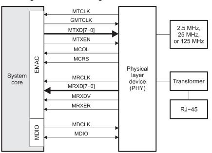
Figure 4. Ethernet Configuration with GMII Interface
