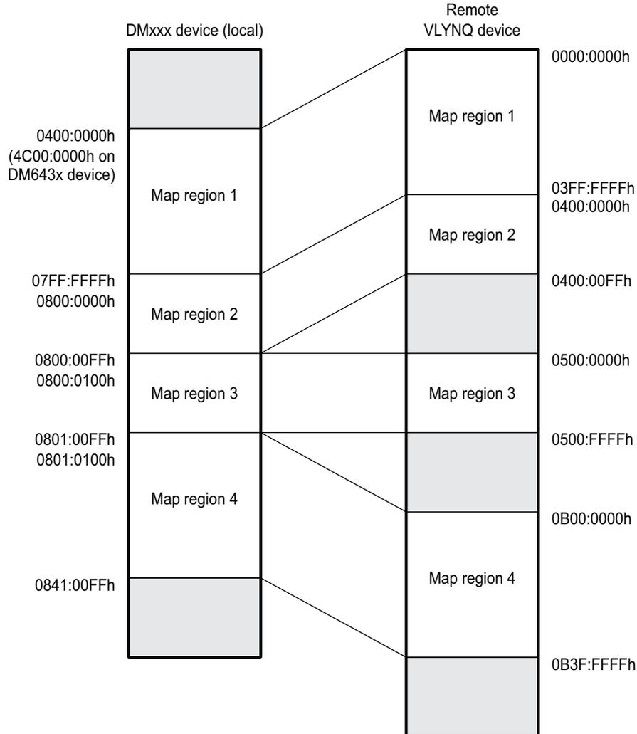
The following shows an example illustrating the address translation used in each VLYNQ module.
