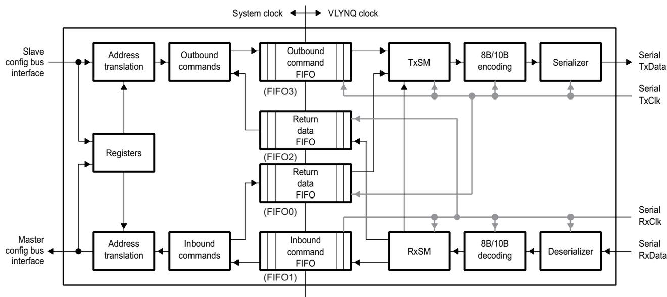
The VLYNQ core module implements two 32-bit configuration bus interfaces. Transmit operations and control register access require the slave configuration bus interface. The master configuration bus interface is required for receive operations. Converting to and from the 32-bit bus to the external serial interface requires serializer and deserializer blocks.
