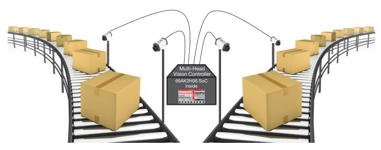
Figure 2 – Example of 66AK2H06 SoC used as the main processor in a multi-head vision controller used to control multiple cameras and run analytics in an industrial automation system
