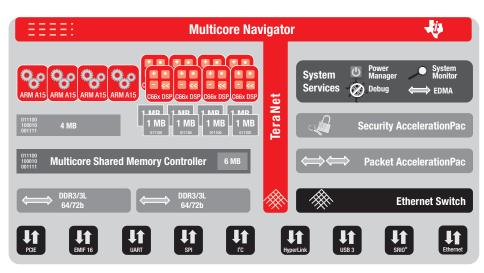
▲ Figure 1 – TI's 66AK2H12 SoC with four Cortex-A15 processors and eight C66x DSP cores
