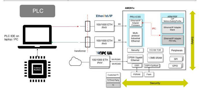
Figure 5-1. Ethernet/IP Solution Using AM261x
