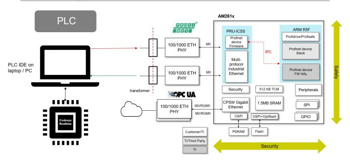
Figure 3-1. Profinet Solution Using AM261x
