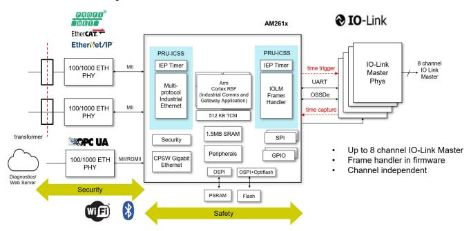
Figure 6-1. IO-LINK Solution Using AM261x
