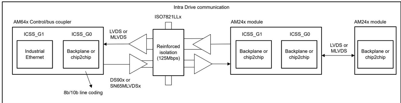
**Figure 2-10. Intra Drive Communication Block Diagram With LVDS Interface and PRU**
