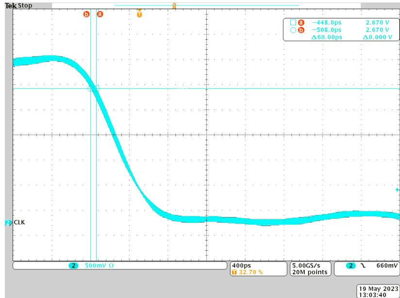
**Figure 4-3. PRU GPO Jitter on Falling Edge**
