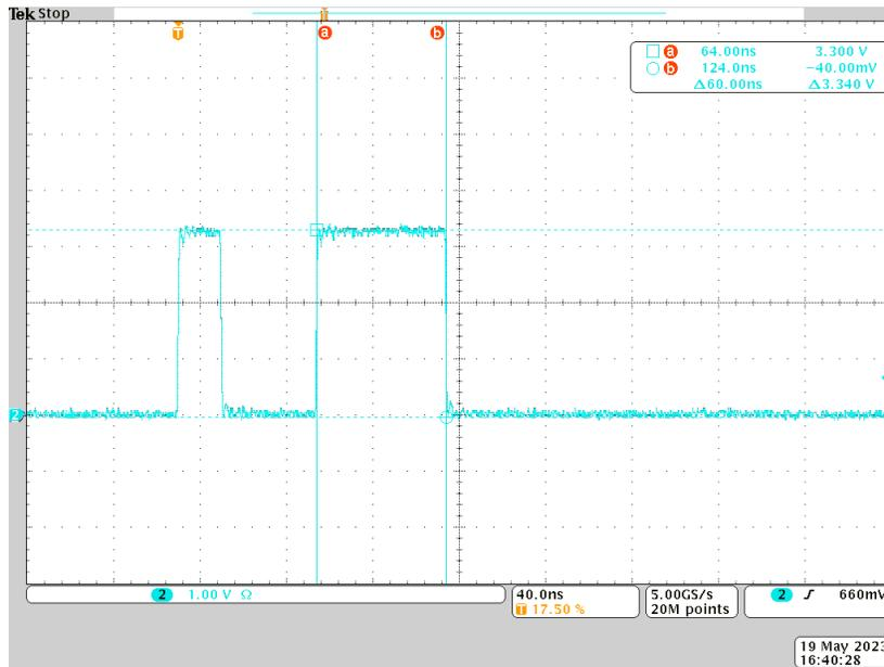
Figure 4-6. Processing Time for 10-bit Data Decoding
