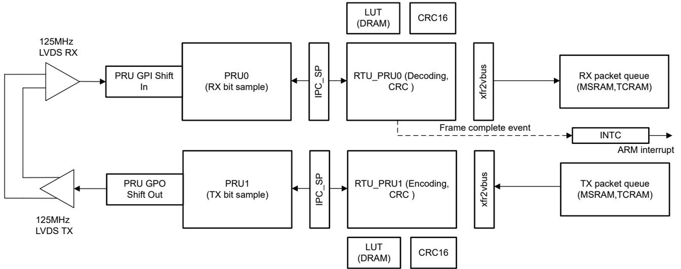
**Figure 3-5. System Block Diagram With PRU and RTU Cores**
