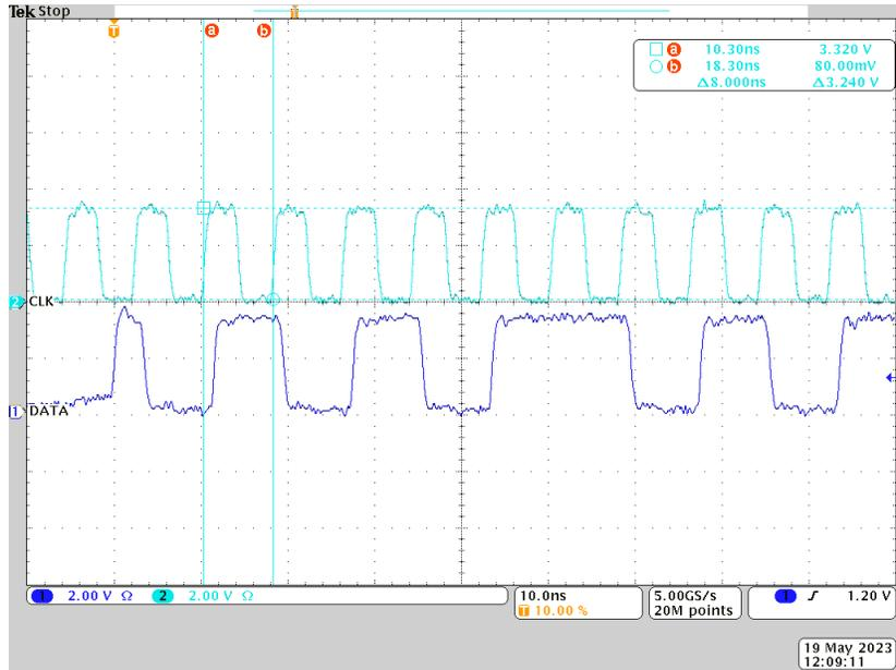
Figure 4-1. Transmitting Data Rates
