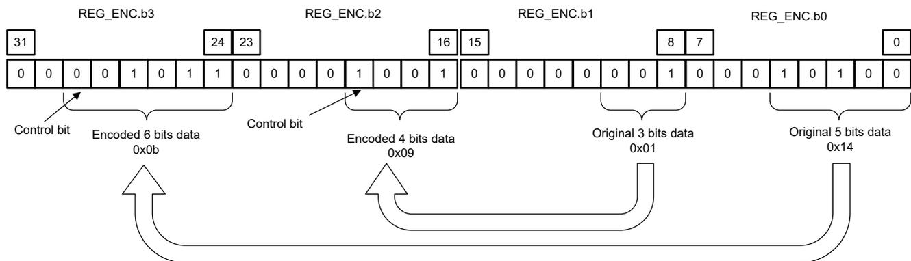
**Figure 2-1. REG\_ENC Encoding Register Distribution**
