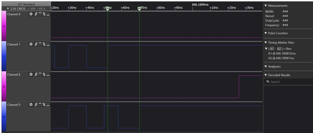
**Figure 2-11. 18ns Latency for DS90LV049 and ISO7821LL LVDS Interfaces**
