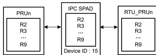
Figure 4-7. Integration of the PRU and IPC Scratch Pad
