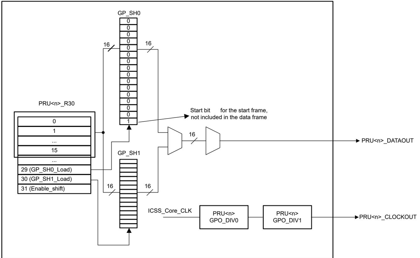
**Figure 2-4. PRU Shift-out Mode Block Diagram**
