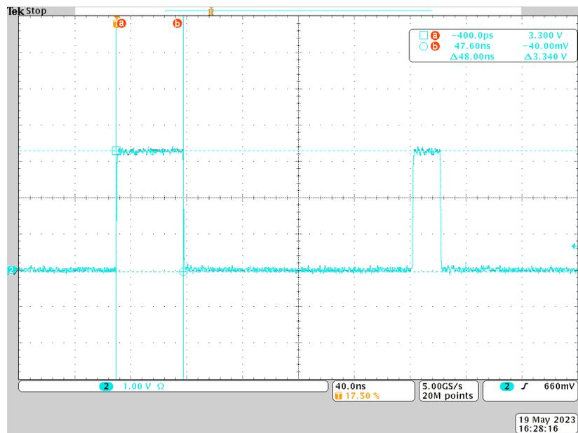
**Figure 4-4. Processing Time for 8-bit Data Encoding**
