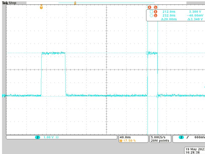
Figure 4-5. Processing Time for CRC16
