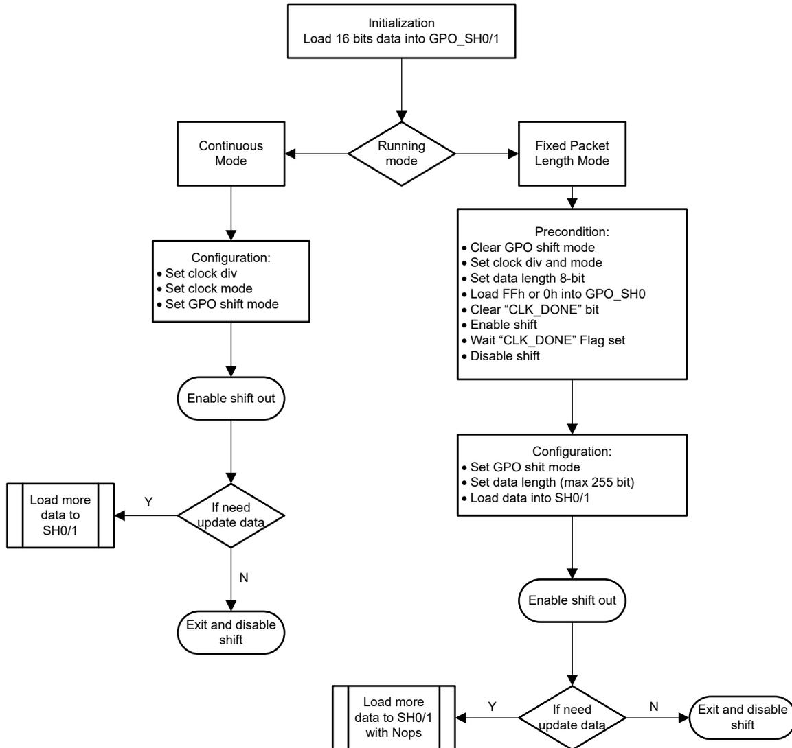
**Figure 2-5. Programming Model of PRU Shift-out Mode**
