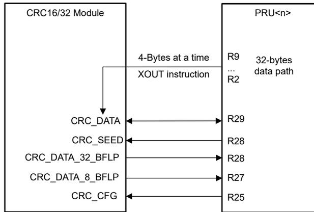
**Figure 3-1. PRU CRC16/32 Module Block Diagram**
