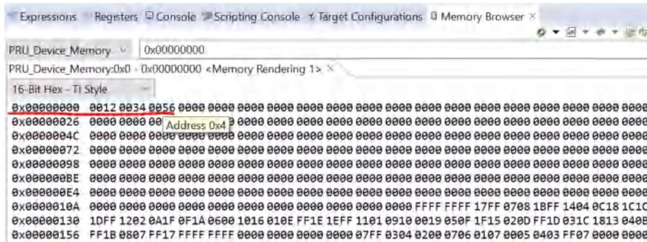
**Figure 2-8. Verification of Data Transmitting With PRU GPIO Shift Mode**
