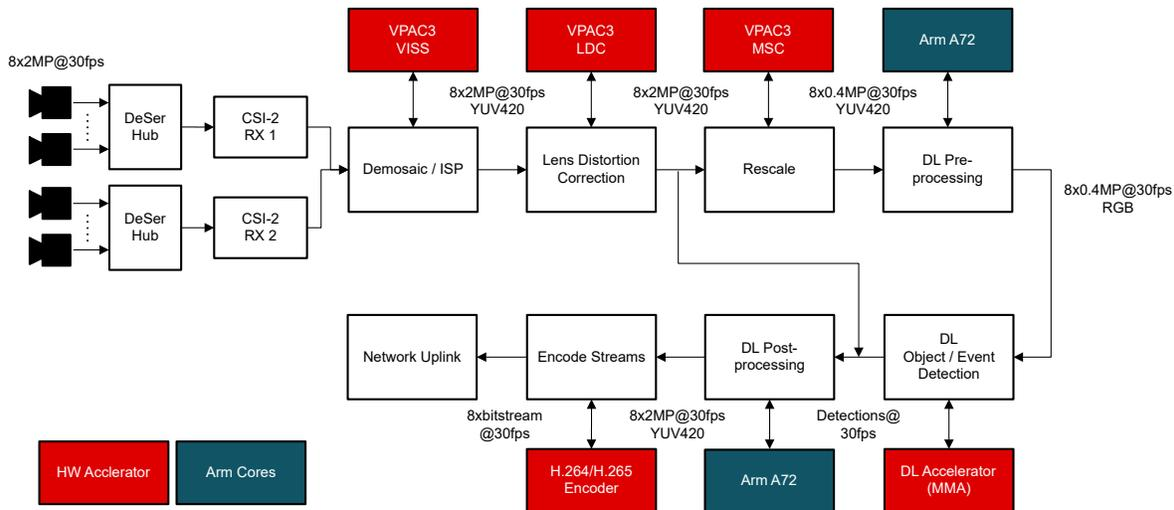
Figure 3-3. Multi-Camera AI Block Diagram With Data Flow on AM69A
