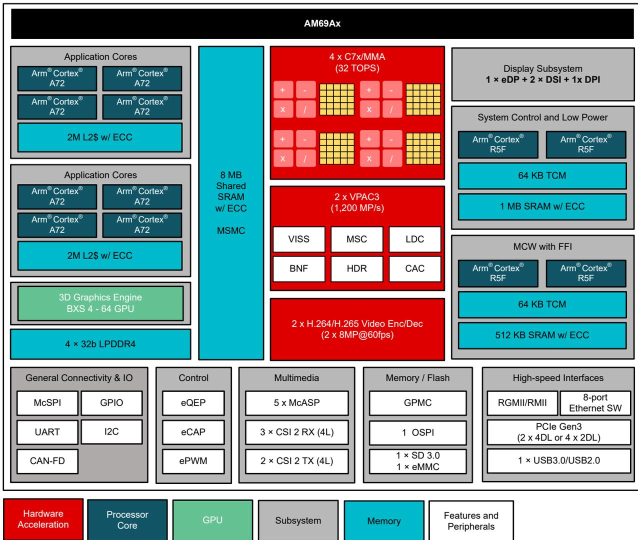
**Figure 2-1. AM69A Block Diagram With Subsystems**
