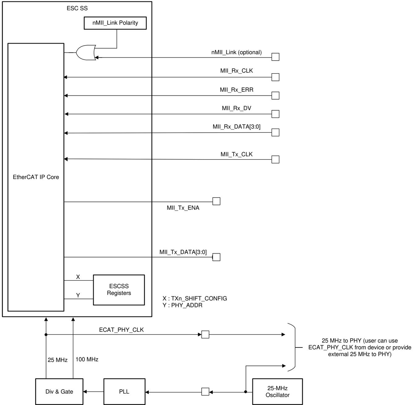
**Figure 2-3. ESC PHY MII Interface Diagram**
