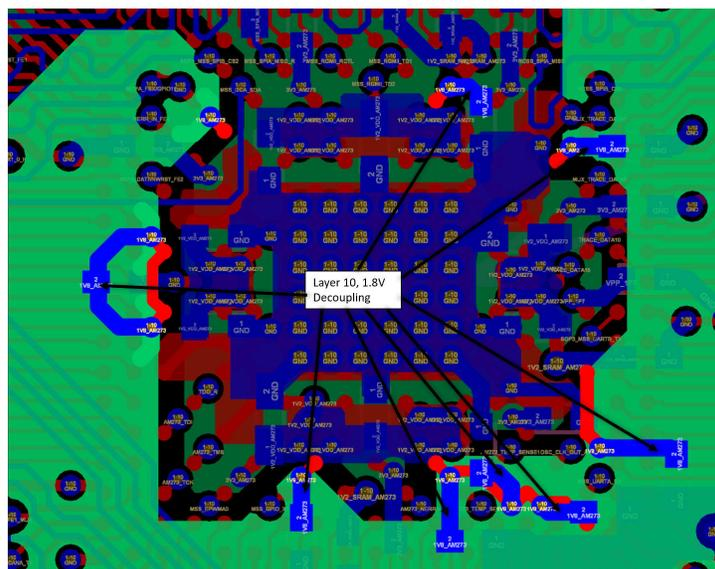
Figure 11-23. AM273 GPEVM Excerpt – 1.8 V Power Decoupling on Layer 10
