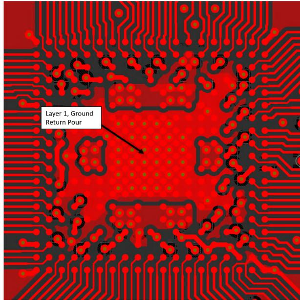
Figure 11-3. ZCE 4 Layer Example Excerpt – Ground Return Pour and Vias Under AM273x BGA Layer 1
