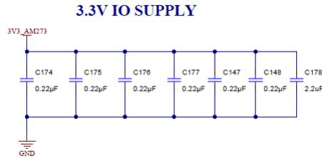
Figure 2-6. AM273x GPEVM Excerpt – 3.3 V Digital I/O Decoupling Schemati
