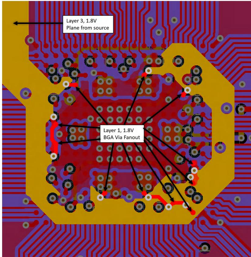
Figure 11-24. ZCE 4 Layer Example Excerpt – 1.8 V Power Via Fan-Out and Plane Routing Layer 3
