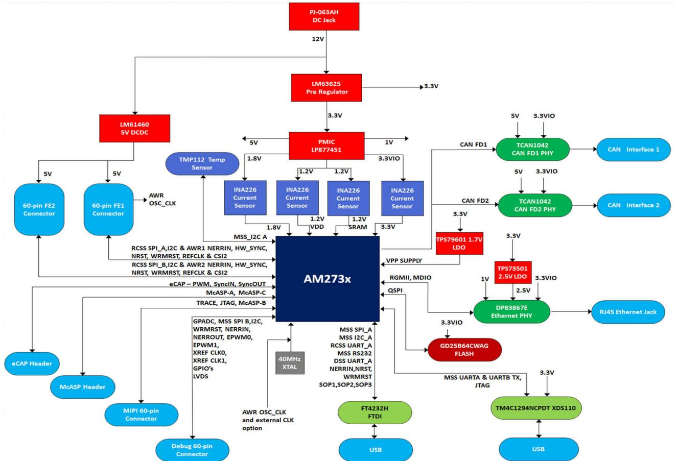
Figure 1-1. Typical AM273x System Block Diagram (Based on TMDS273GPEVM Design)
