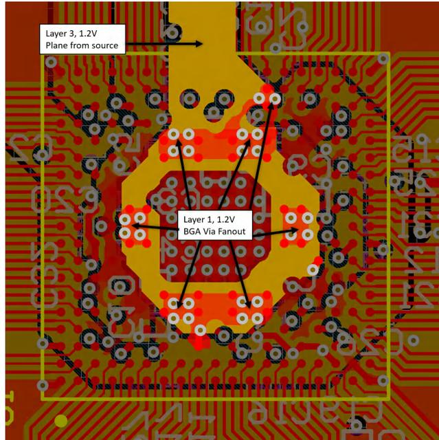
Figure 11-10. ZCE 4 Layer Example Excerpt – 1.2 V Core Power Output From Source and BGA Vias
