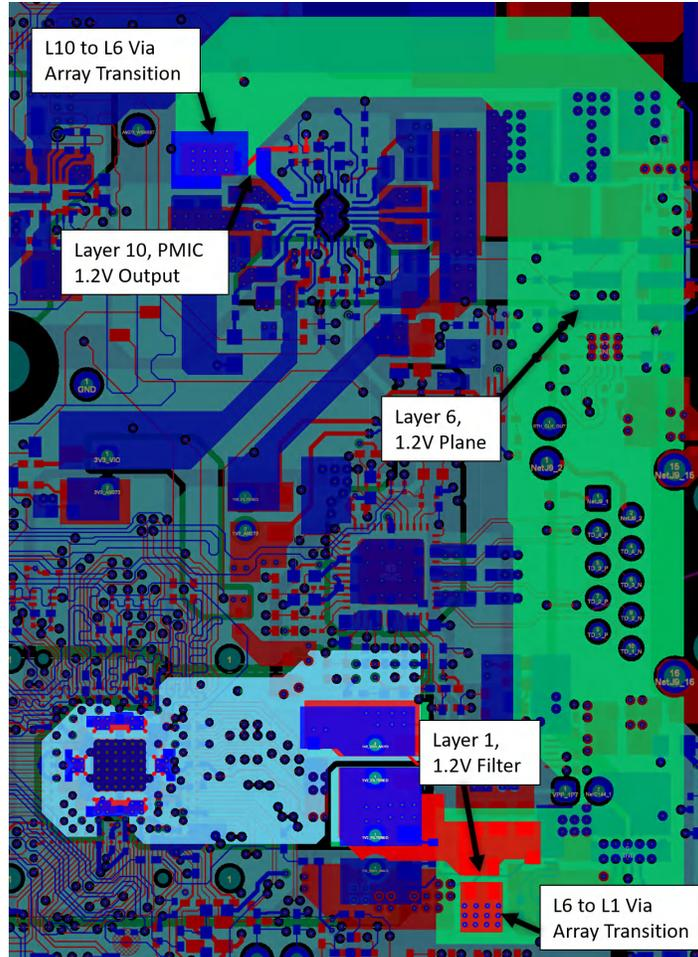
**Figure 11-7. AM273 GPEVM Excerpt – 1.2 V Core Power Output from PMIC, Power Plane Vias, and BGA Vias**
