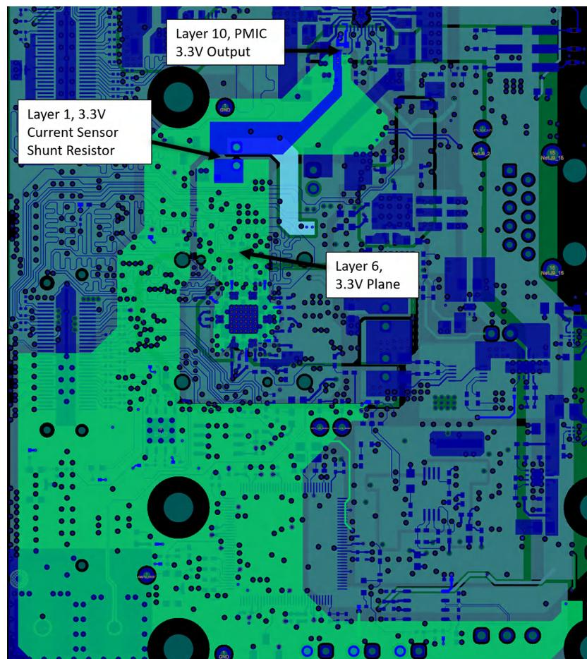
**Figure 11-14. AM273 GPEVM Excerpt – 3.3 V Digital and Analog Power Planes on Layer 6**
