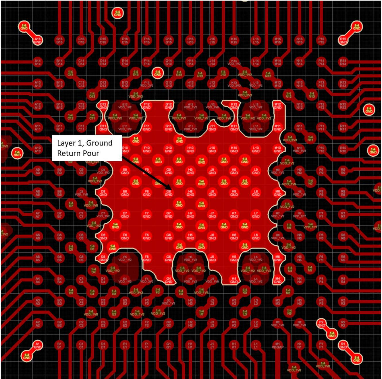
Figure 11-5. NZN 4 Layer Example Excerpt – Ground Return Pour and Vias Under AM273x BGA Layer 1
