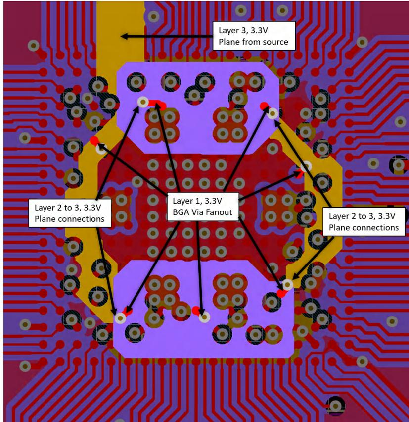
**Figure 11-17. ZCE 4 Layer Example Excerpt – 3.3 V Digital and Analog Power Planes on Layers 2 and 3 and BGA Vias**
