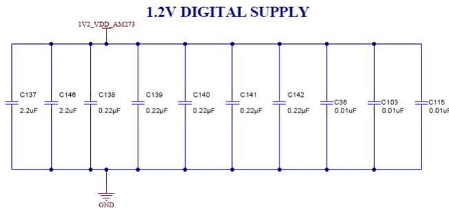
**Figure 2-4. AM273x GPEVM Excerpt – 1.2 V Power Decoupling Schematic**
