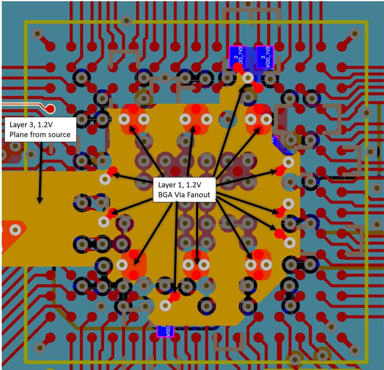
Figure 11-12. NZN 4 Layer Example Excerpt – 1.2 V Core Power Output from source and BGA Vias
