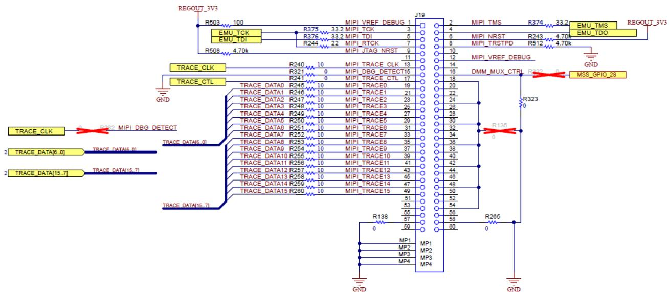
**Figure 6-1. Example MIPI-60 JTAG and 16-Bit Trace Implementation**
