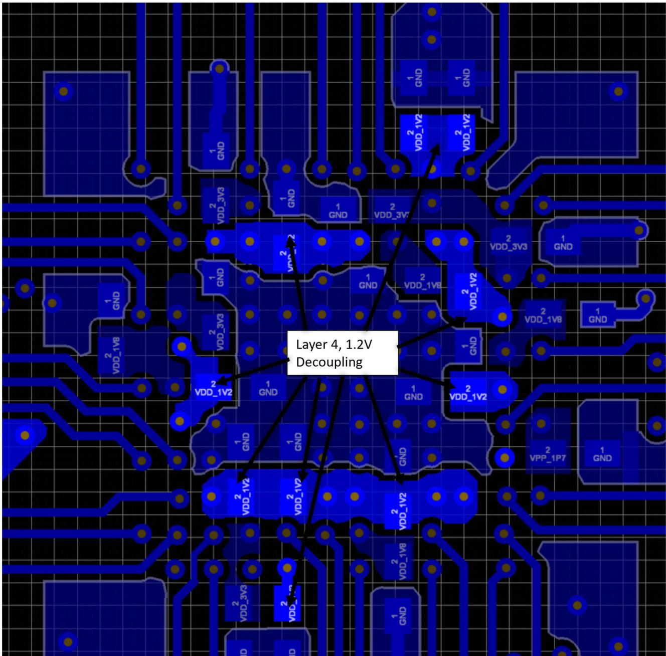
Figure 11-13. NZN 4 Layer Example Excerpt – 1.2 V Core Power Decoupling Mounting, Layer 4
