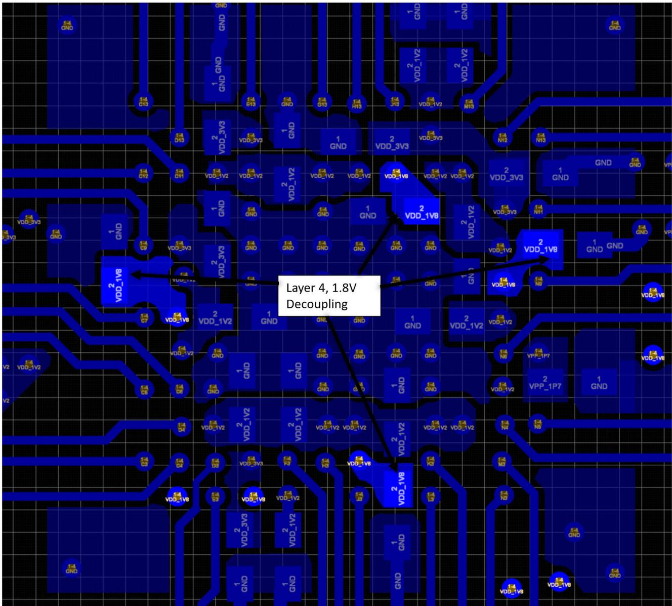
Figure 11-27. NZN 4 Layer Example Excerpt – 1.8 V Power Decoupling on Layer 4
