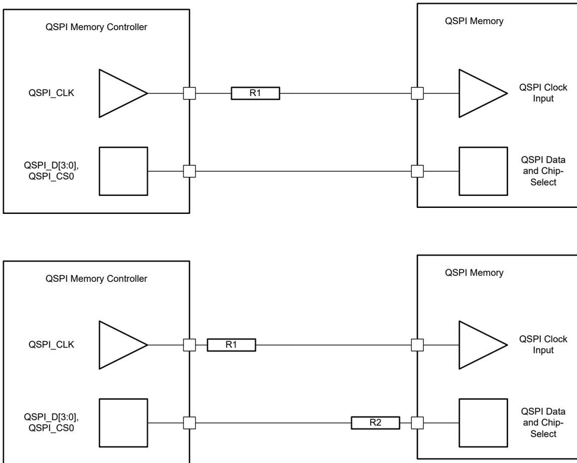
**Figure 5-3. AM273x QSPI - Routing Rules Diagram**
