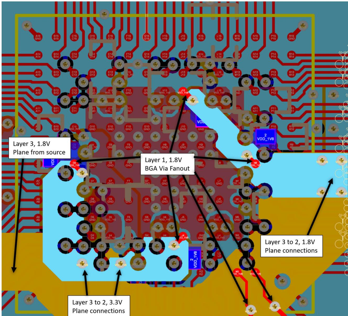
Figure 11-26. NZN 4 Layer Example Excerpt – 1.8 V Power Via Fan-Out and Plane Routing Layer 3
