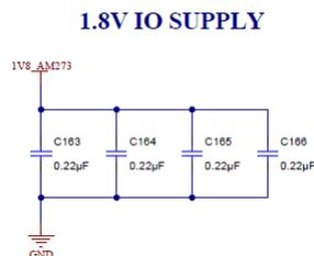
**Figure 2-5. AM273x GPEVM Excerpt – 1.8 V Digital I/O Decoupling Schematic**
