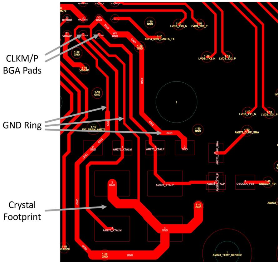
Figure 3-2. Excerpt From AM273x GPEVM Layout - Crystal Layout and Ground Ring Structure
