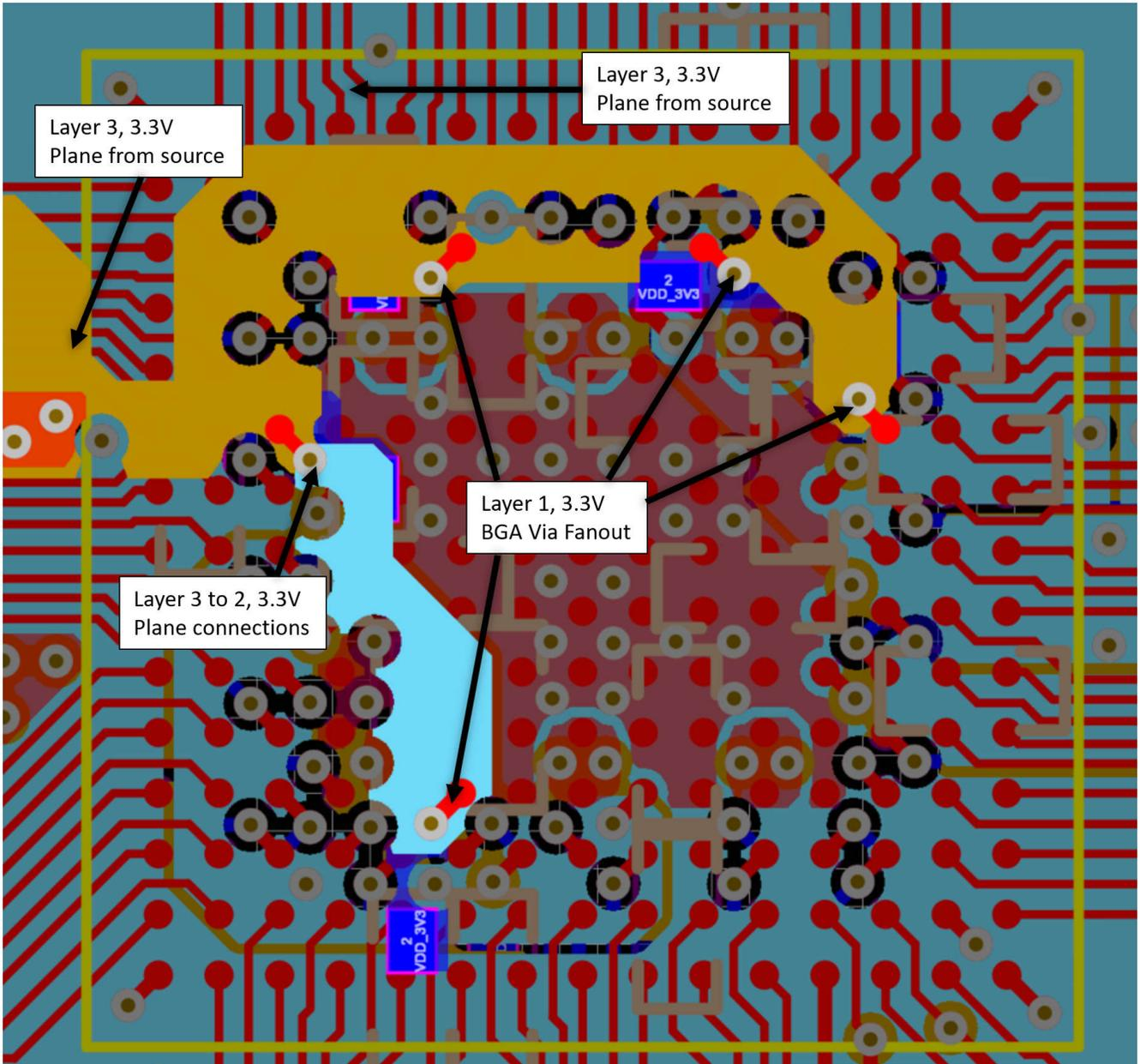
Figure 11-19. NZN 4 Layer Example Excerpt – 3.3 V Digital and Analog Power Planes on Layers 2 and 3 and BGA Vias
