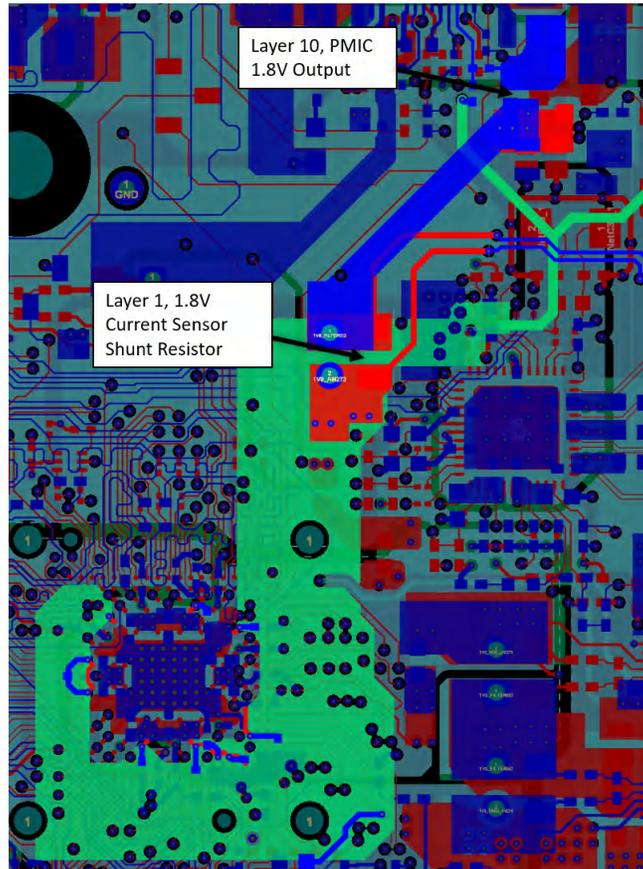
Figure 11-21. AM273 GPEVM Excerpt – 1.8 V Digital Power Via Fan-Out and Plane Routing Layer 6
