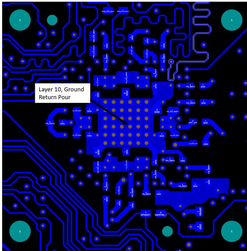
Figure 11-2. AM273 GPEVM Excerpt – Ground Return Pour and Vias Under AM273x BGA Layer 10
