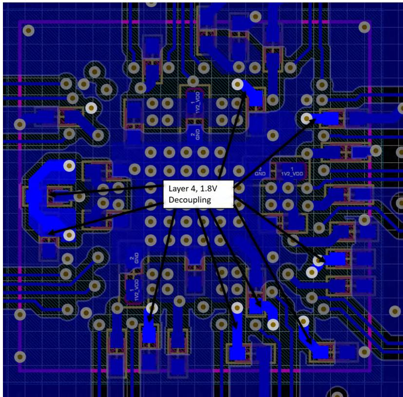
Figure 11-25. ZCE 4 Layer Example Excerpt – 1.8 V Power Decoupling on Layer 4
