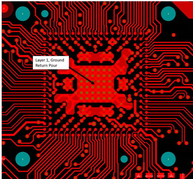
Figure 11-1. AM273 GPEVM Excerpt – Ground Return Pour and Vias Under AM273x BGA Layer 1
