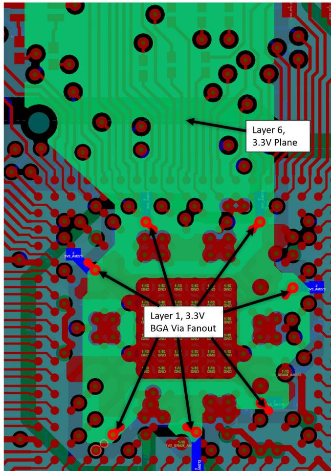
Figure 11-15. AM273 GPEVM Excerpt – 3.3 V Digital I/O and Analog I/O BGA Pinout
