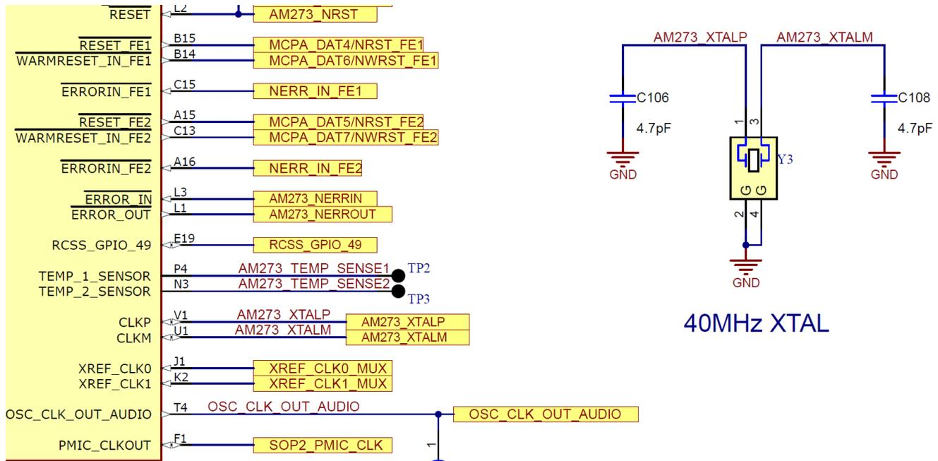
**Figure 3-1. Excerpt From AM273x GPEVM Schematics**
