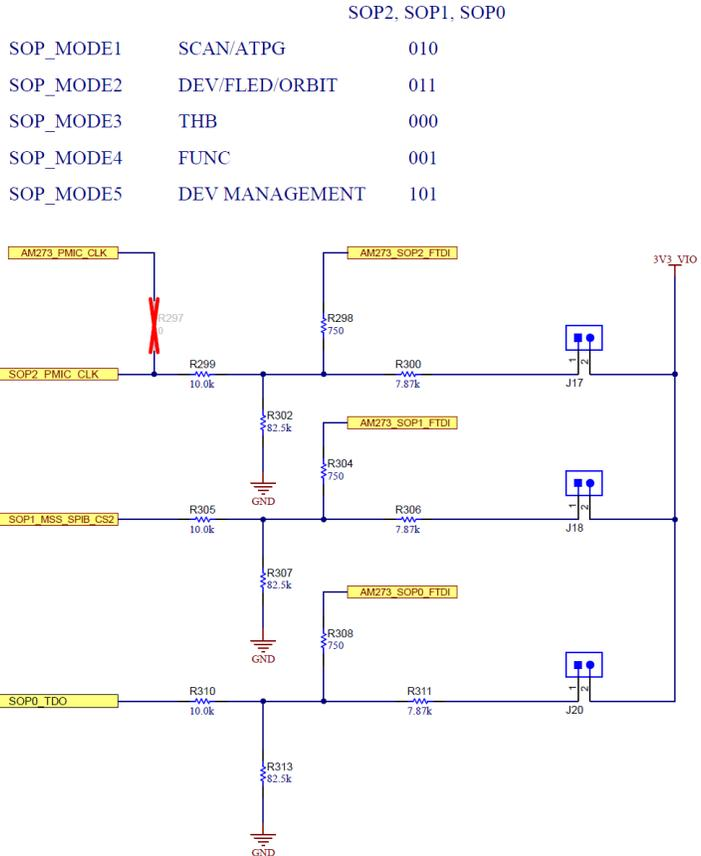
Figure 5-1. Excerpt From AM273x GPEVM Schematic – SOP[4:0] Functional and SOP Paths
