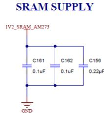
Figure 2-7. AM273x GPEVM Excerpt – SRAM Decoupling Schematic
