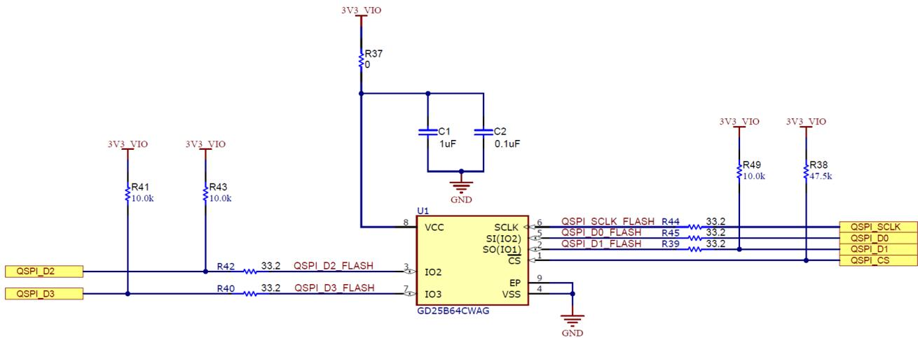
**Figure 5-2. Excerpt From AM273x GPEVM Schematic – AM273x QSPI Controller and GD25B64CWAG NOR Flash Memory**
