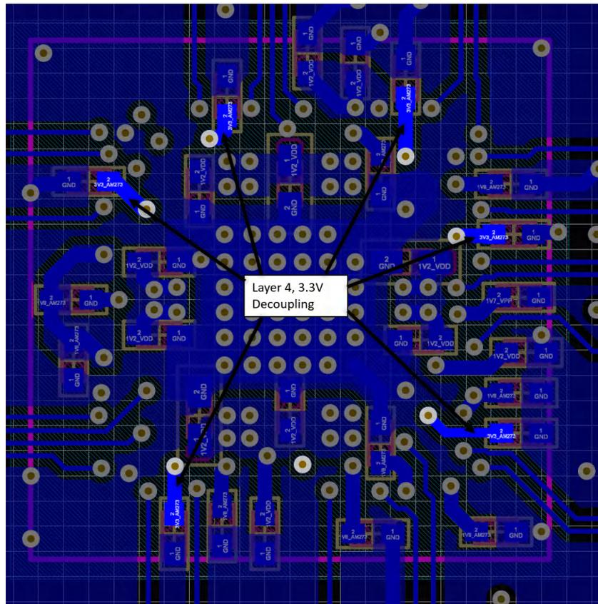
**Figure 11-18. ZCE 4 Layer Example Excerpt – 3.3 V Decoupling**
