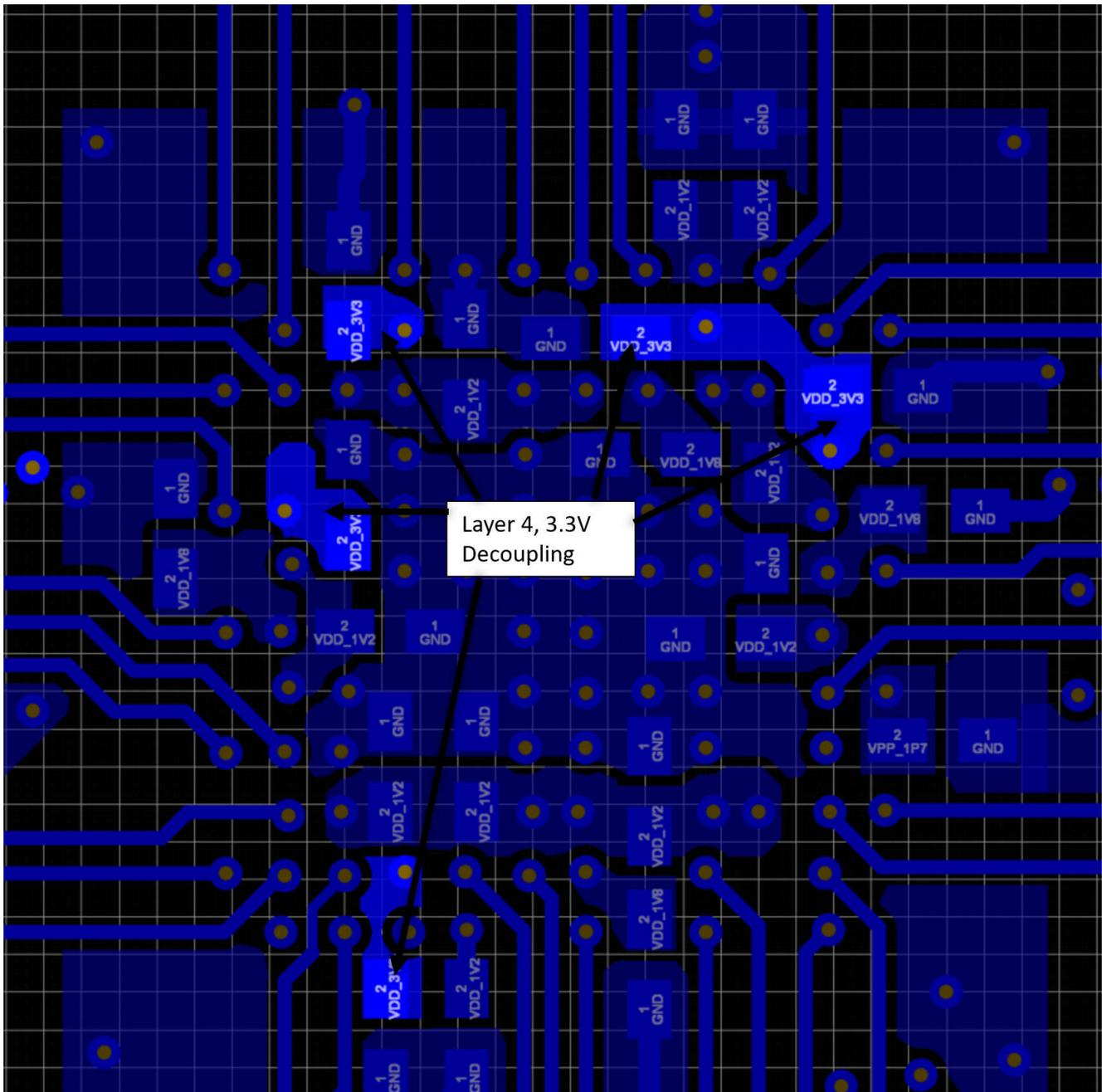
Figure 11-20. NZN 4 Layer Example Excerpt – 3.3 V Decoupling
