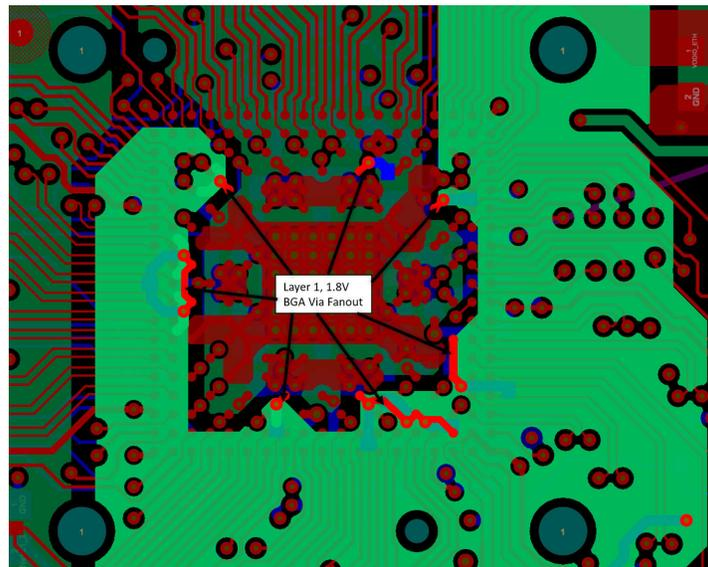
Figure 11-22. AM273 GPEVM Excerpt – 1.8 V Power Via Fan-Out and Plane Routing Layer 6
