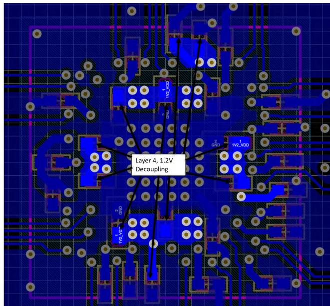
Figure 11-11. ZCE 4 Layer Example Excerpt – 1.2 V Core Power Decoupling Mounting, Layer 4
