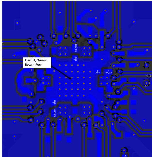
Figure 11-4. ZCE 4 Layer Example Excerpt – Ground Return Pour and Vias Under AM273x BGA Layer 4
