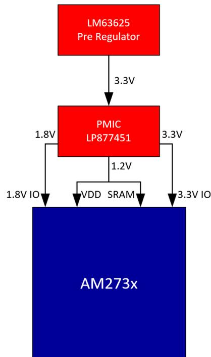
**Figure 2-1. AM273x PMIC Example Solution**
