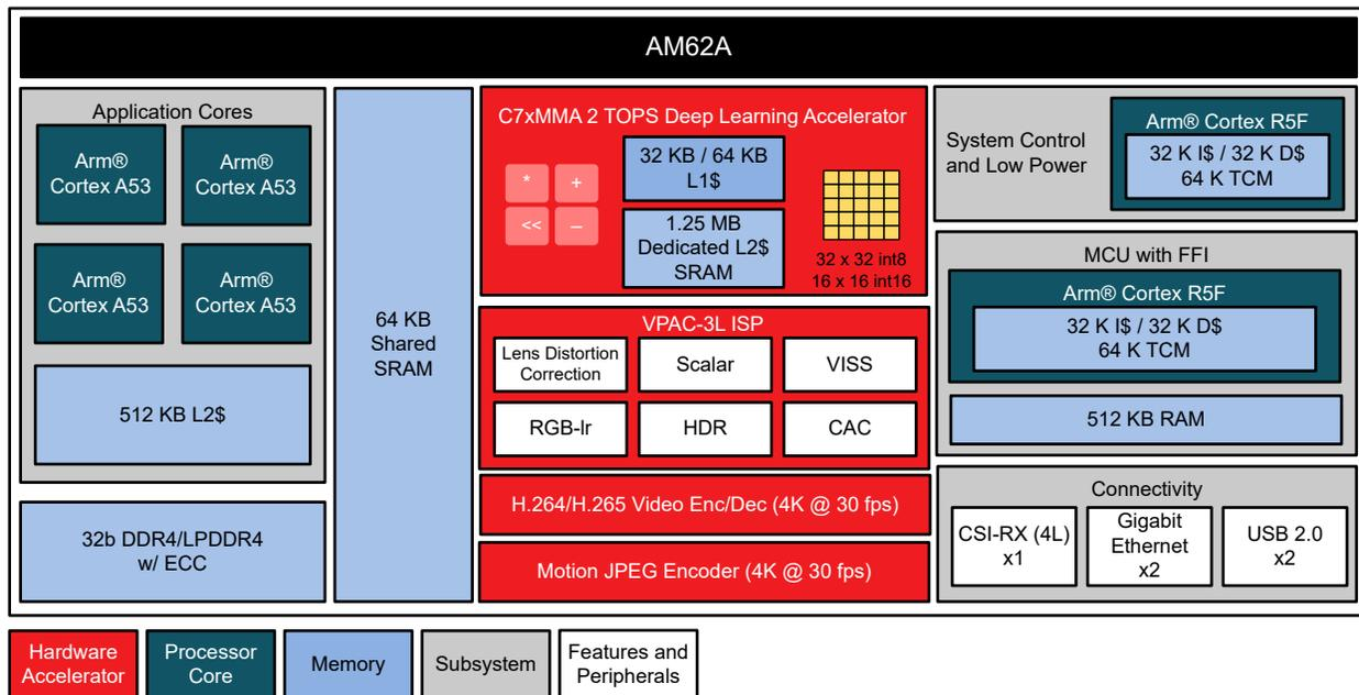
**Figure 2. AM62A SoC Simplified Block Diagram**
