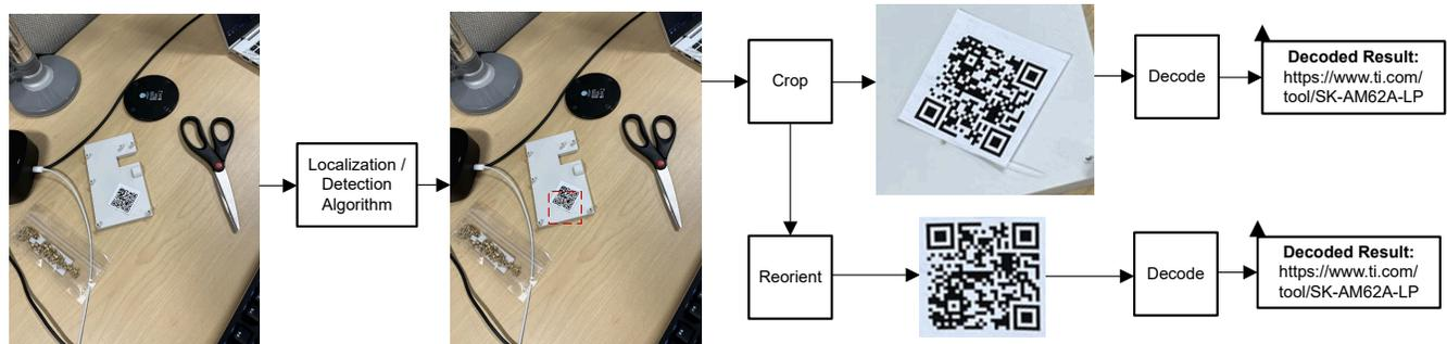
Figure 1. Application Dataflow for Barcode Reader
