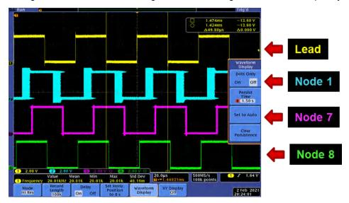
Figure 7-12. 1 Lead - 8 Node Device Without EPWM Synchronization
