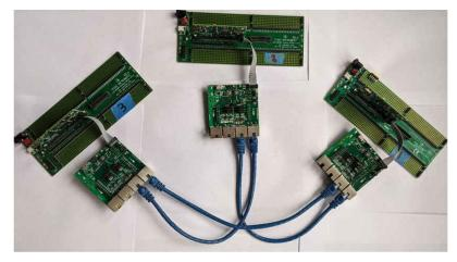
Figure 5-6. Test Platform for Three Devices Communication
