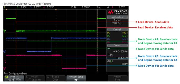
Figure 5-7. FSI Communication With CPU Control Among Three Devices
