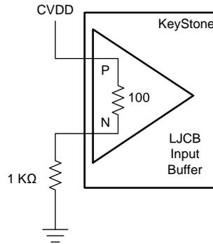
**Figure 3. Unused LJCB Clock Input Connection**
