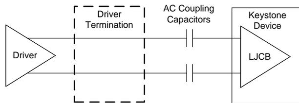
Figure 1. LJCB Differential Clock Inputs
